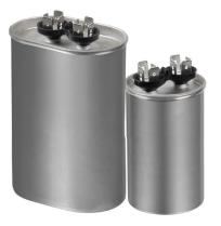
Type SF, AC rated metallized polypropylene capacitors provide starting torque and power factor correction for split phase motors typically used in refrigeration and air conditioning motorrun applications. Type SF also may be used to provide noise suppression, voltage regulation and line current reduction in power supply applications.
