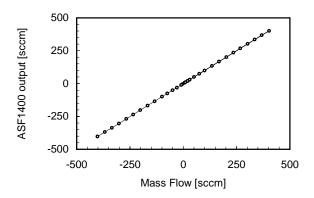
Figure 2: ASF1400 transfer characteristics.
