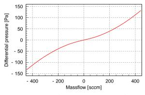
Figure 4: Differential Pressure vs. Mass Flow of ASF1400 Device.
