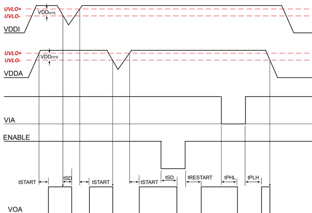
Figure 2.18. Device Behavior during Normal Operation and Shutdown
