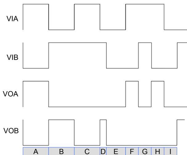
**Figure 2.19. Input / Output Waveforms for Si8273 Drivers**
