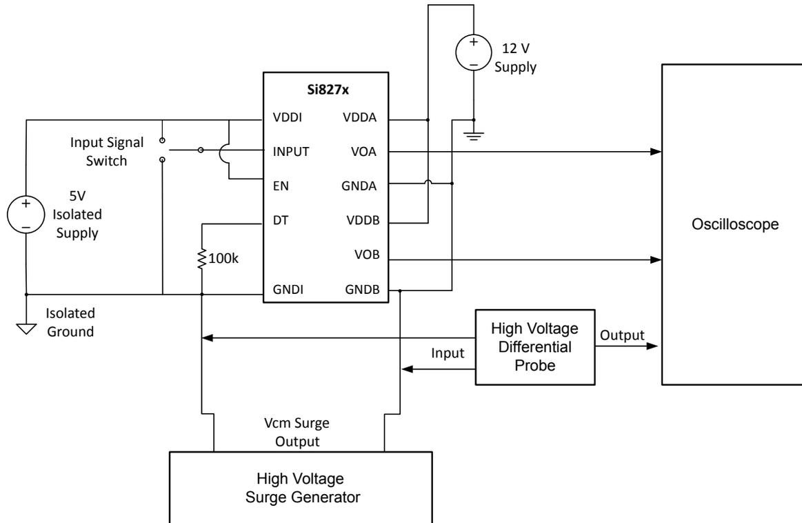
Figure 4.3. Common Mode Transient Immunity Test Circuit
