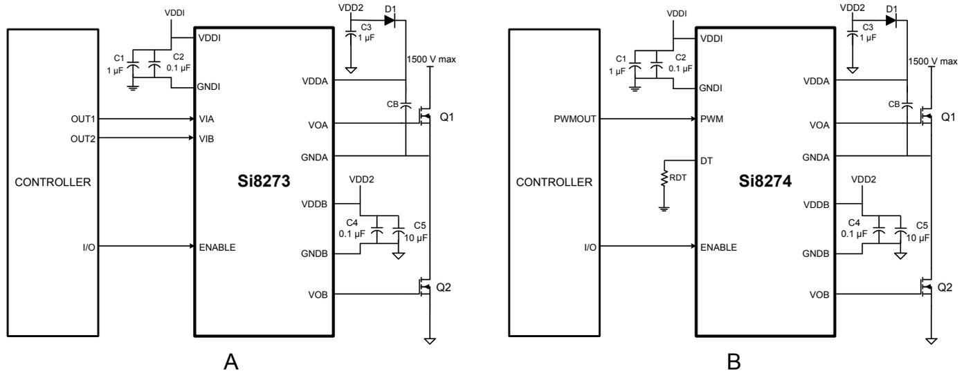
**Figure 3.1. Si827x in Half-Bridge Application**
