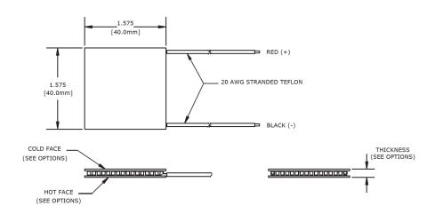
Ceramic Material: Alumina (Al<sub>2</sub>O<sub>2</sub>)
