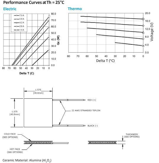
Ceramic Material: Alumina (Al<sub>2</sub>O<sub>3</sub>) Solder Construction: 232°C, Tin Antimony (SnSb)
