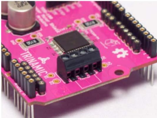
For an experimental setup it is recommended to use the provided screw terminals. But you can use anything that fits into the holes as long as it withstands the current for your motor (better be on the safe side and use a connector rated for at least 2A)
