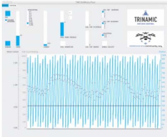
In the main screen you can adjust all basic parameters of the TMC260 driver chip. Let's go through them in order to start you motor:
