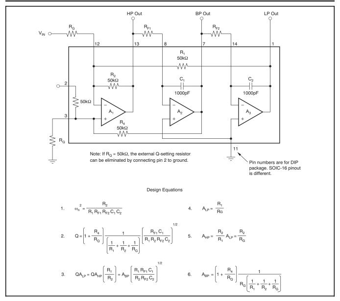
Figure 2. Inverting Pole-Pair
