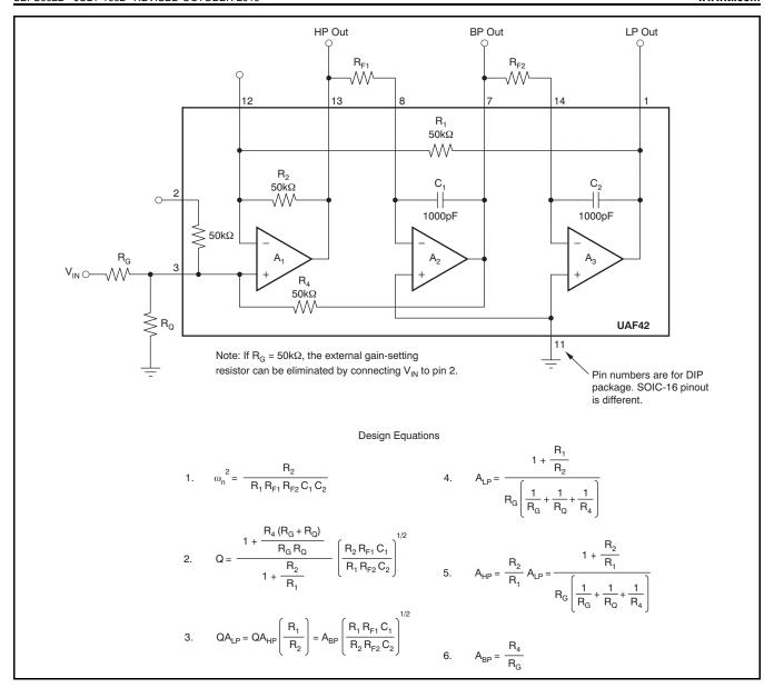
Figure 1. Noninverting Pole-Pair
