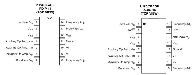
NOTE: (1) NC = no connection. For best performance connect all *NC* pins to ground to minimize inter-lead capacitance.
