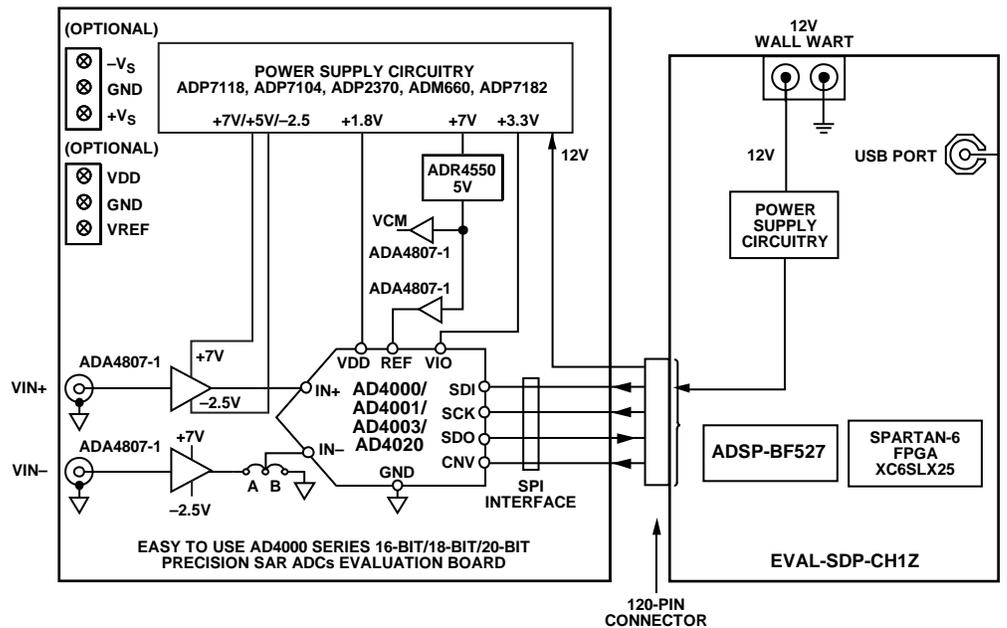
Figure 2. Simplified Evaluation Board Block Diagram
