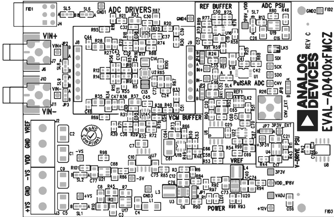
Figure 29. ADC Evaluation Board Silkscreen, Top Layer
