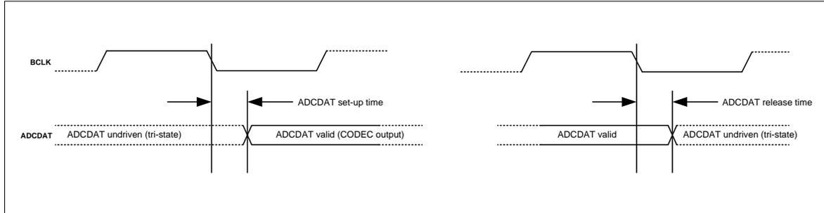
**Figure 4 Audio Interface Timing - TDM Mode**
