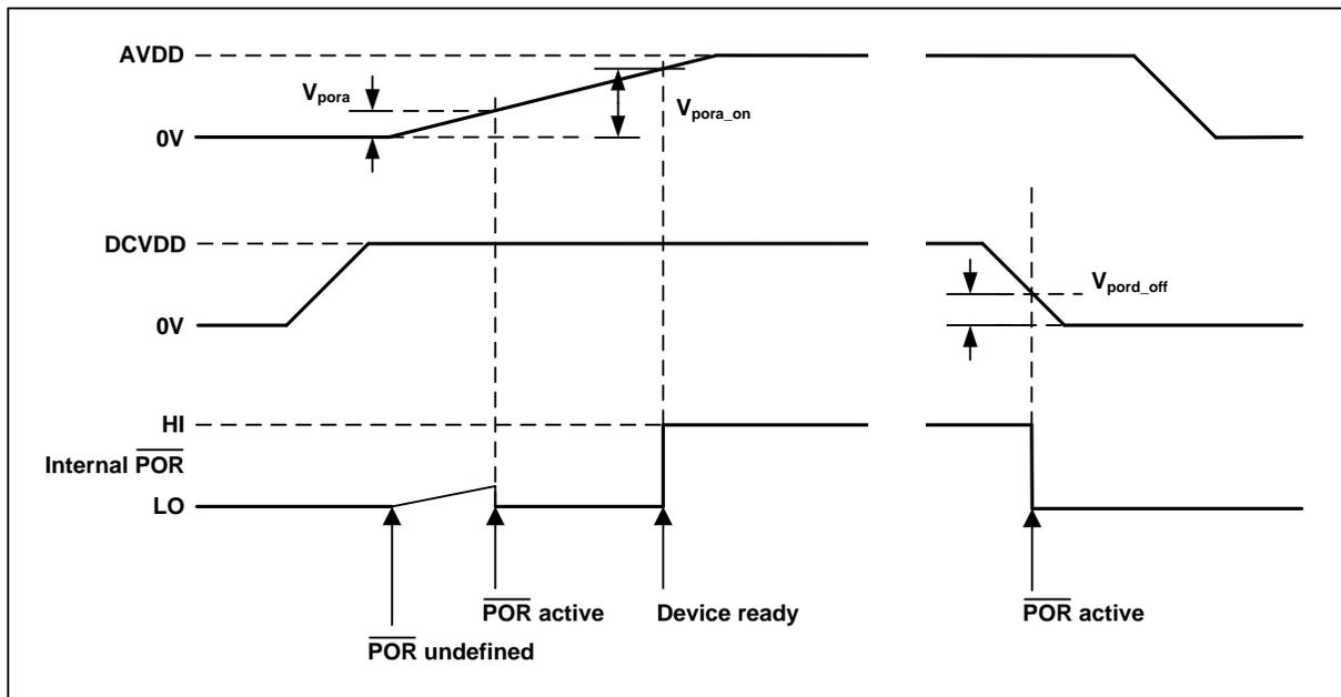
**Figure 70 Power On Reset timing - DCVDD enabled first**
