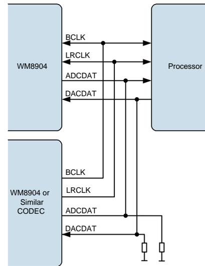
**Figure 43 TDM with Other CODEC as Master**
