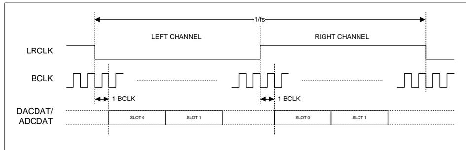
**Figure 54 TDM in I<sup>2</sup>S Mode**
