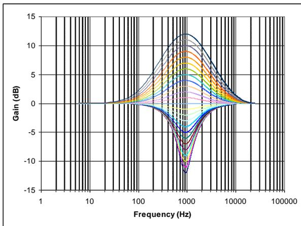
**Figure 32 EQ Band 3 – Peak Filter Response**
