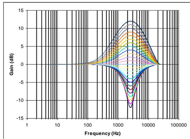
**Figure 33 EQ Band 4 – Peak Filter Response**
