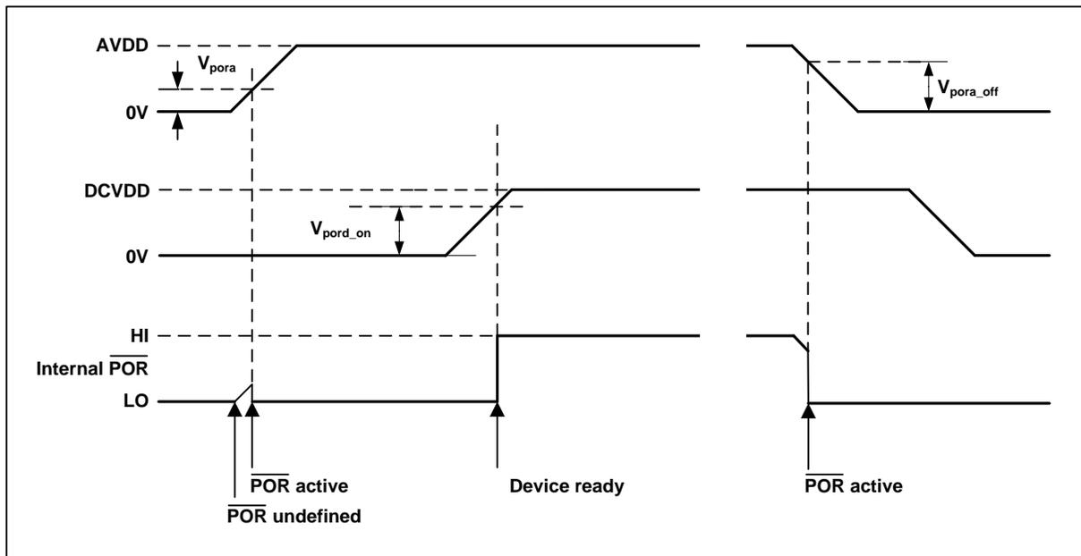
**Figure 69 Power On Reset timing - AVDD enabled first**
