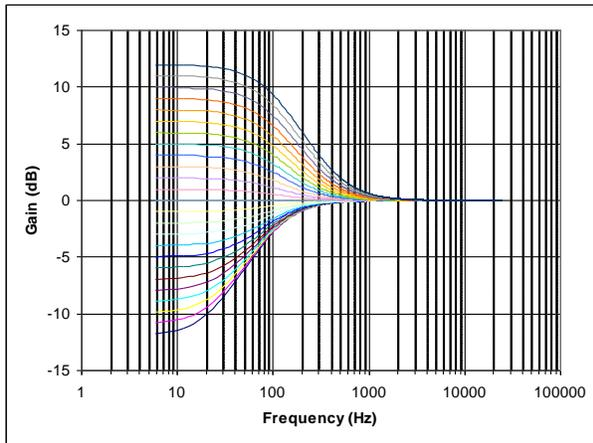
**Figure 30 EQ Band 1 – Low Freq Shelf Filter Response**
