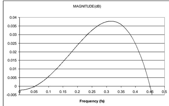
**Figure 11 DAC Digital Filter Ripple (Normal Mode)**
