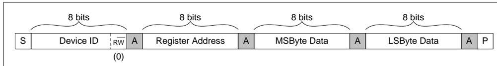
**Figure 63 Single Register Write to Specified Address**
