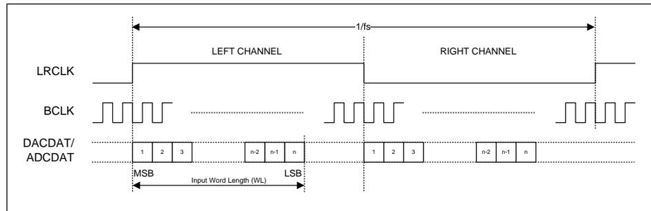
**Figure 46 Left Justified Audio Interface (assuming n-bit word length)**
