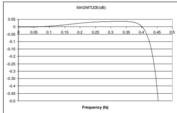
**Figure 13 DAC Digital Filter Ripple (Sloping Stopband Mode)**
