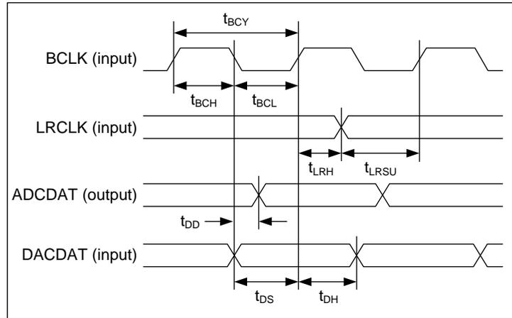
**Figure 3 Audio Interface Timing – Slave Mode**
