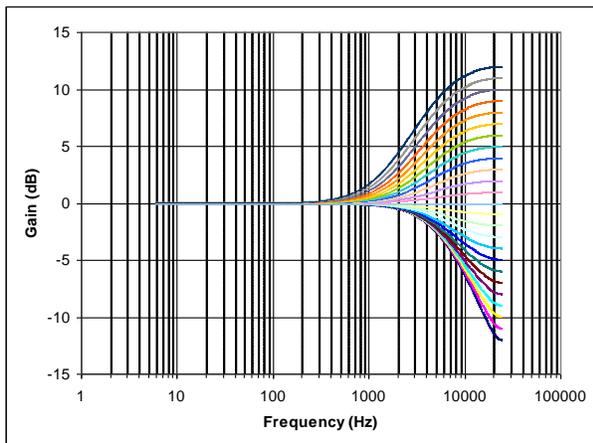
**Figure 34 EQ Band 5 – High Freq Shelf Filter Response**
