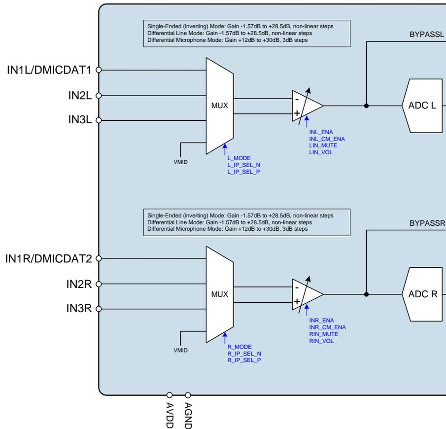
Figure 20 Block Diagram for Input Signal Path
