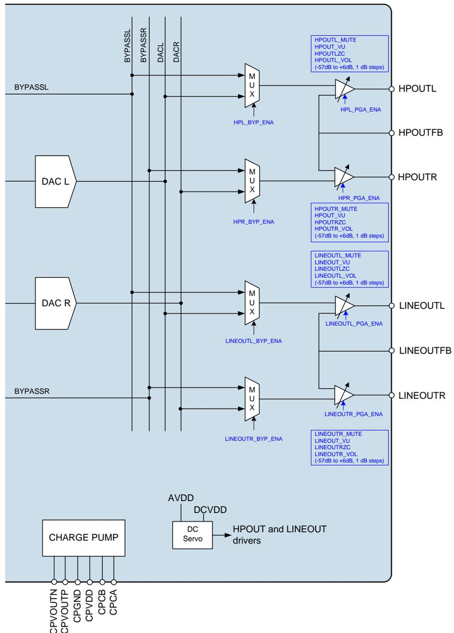
**Figure 37 Output Signal Path and Control Registers**
