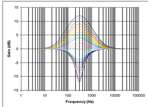
**Figure 31 EQ Band 2 – Peak Filter Response**
