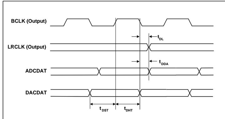
**Figure 2 Audio Interface Timing – Master Mode**
