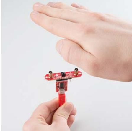
Try out the other tabs in the application! The Z-Control tab lets you try moving your hand toward and away from the sensor, and the Gestures tab computes a few different gestures based on the Z- and X- data.
