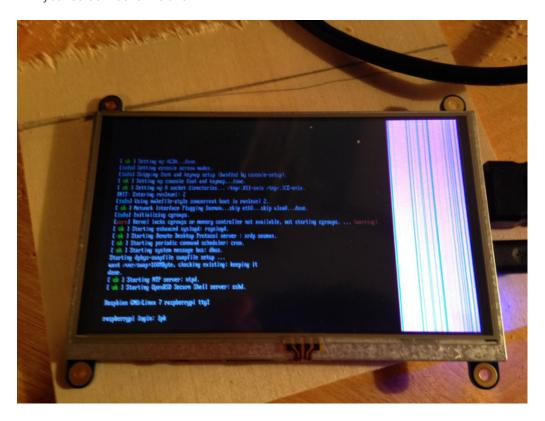
It is not broken - what is happening is you are sending 640x480 data to the monitor but since it does not have a scaler, and the display is 800x480, the remaining 160 pixels are 'not drawn' - you must set the resolution of your computer to 800x480 to get all of the pixels used! For raspberry pi, check the Config page for the correct config.txt setup for 800x480
