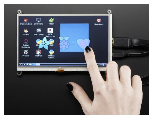
Its a mini HDMI monitor! So small and simple, you can use this display with any computer that has HDMI output, and the shape makes it easy to attach to a case or rail. This backpack features the TFP401 for decoding video, and for the touch version, an AR1100 USB resistive touch screen driver.
