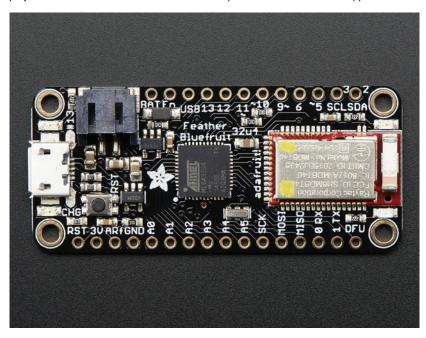
At the Feather 32u4's heart is at ATmega32u4 clocked at 8 MHz and at 3.3V logic, a chip setup we've had tons of experience with a<u>k's the same</u> as the Flora (http://adafru.it/dVI). This chip has 32K of flash and 2K of RAM, with built in USB so not only does it have a USB-to-Serial program & debug capability built in with no need for an FTDI-like chip, it can also act like a mouse, keyboard, USB MIDI device, etc.
