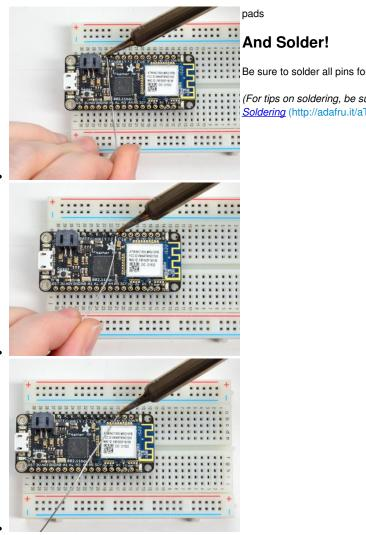
Be sure to solder all pins for reliable electrical contact.
