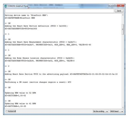
If you open up an application on your mobile device or laptop that support the standard<u>Heart Rate Monitor Service</u> (http://adafru.it/f4l), you should be able to see the heart rate being updated in sync with the changes seen in the Serial Monitor:
