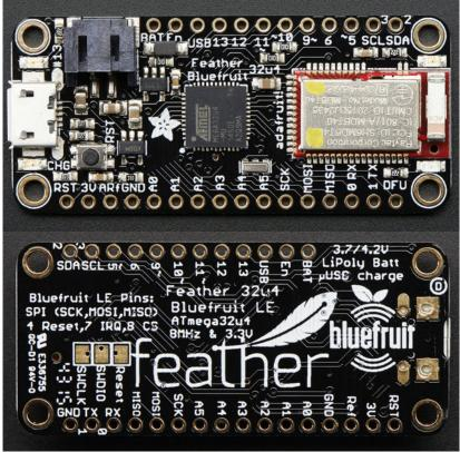
The DFU pin is accidentally labeled GND on the bottom, sorry about that! it should be labeled DFU, dont use it as a GND
