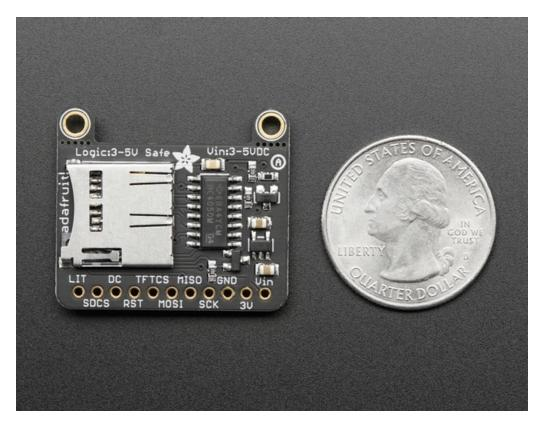
The breakout has the TFT display soldered on (it uses a delicate flex-circuit connector) as well as a ultra-low-dropout 3.3V regulator and a 3/5V level shifter so you can use it with 3.3V or 5V power and logic. We also had a little space so we placed a microSD card holder so you can easily load full color bitmaps from a FAT16/FAT32 formatted microSD card. The microSD card is not included, but you can pick one up here.
