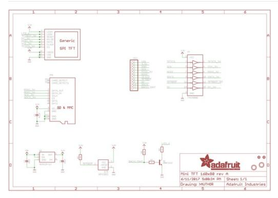
For the level shifter we use the CD74HC4050 which has a typical propagation delay of ~10ns
