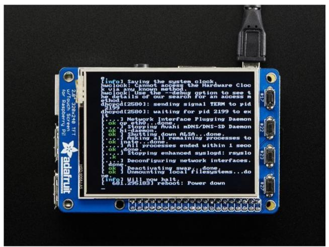
This design uses the hardware SPI pins (SCK, MOSI, MISO, CE0, CE1) as well as GPIO #25 and #24. All other GPIO are unused. Since we had a tiny bit of space, there's 4 spots for optional slim tactile switches wired to four GPIOs, that you can use if you want to make a basic user interface. For example, you can use one as a power on/off button.
