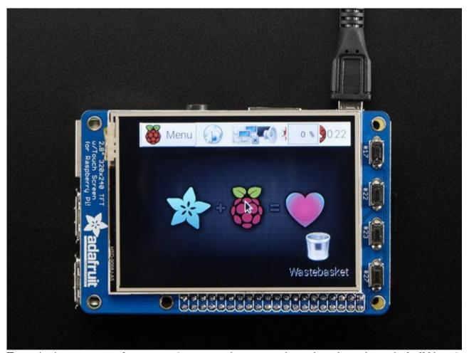
To make it super easy for use: we've created a custom kernel package based of off Notro's awesome framebuffer work, so you can install it over your existing Raspbian (or derivative) images in just a few commands.
