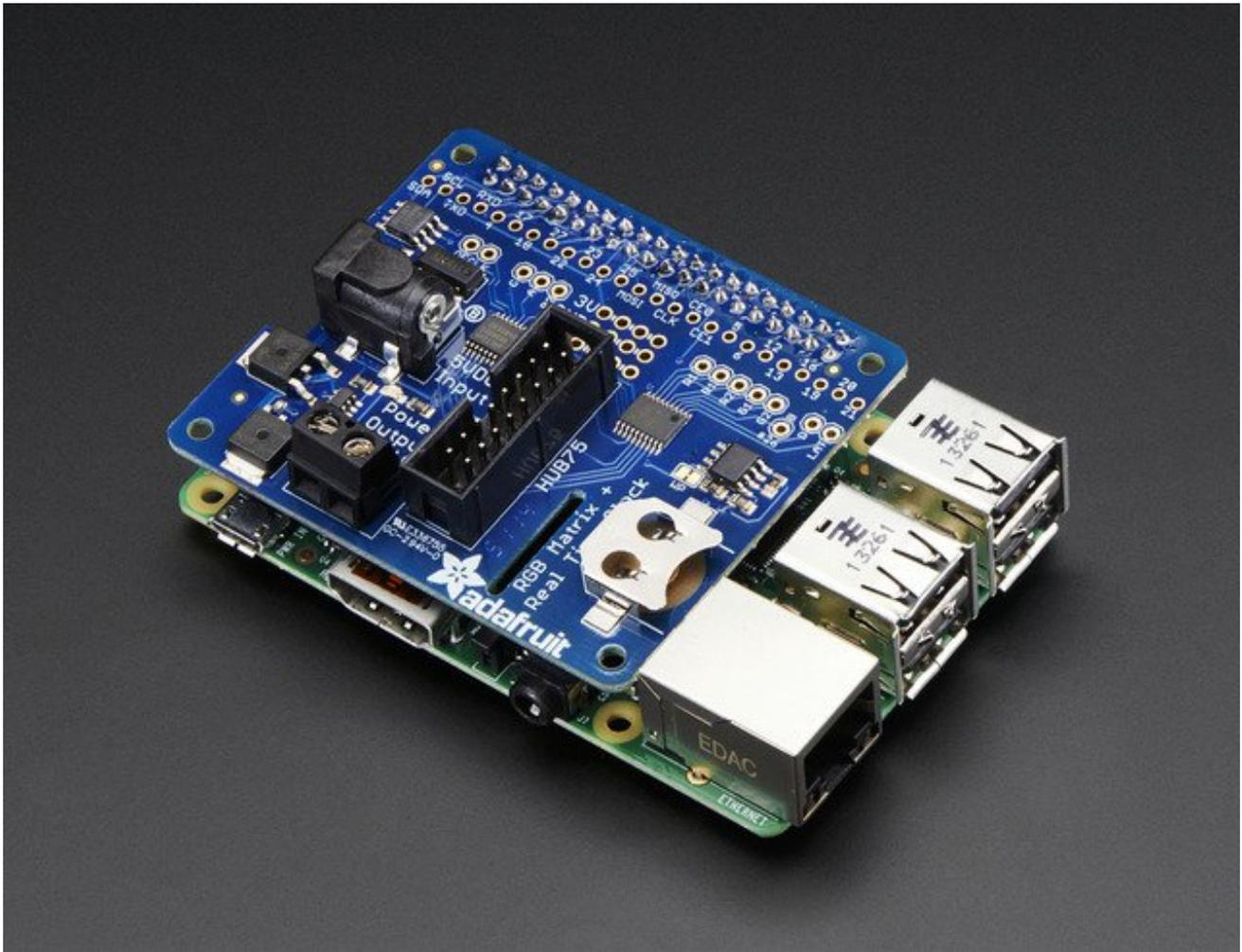
Works with any of our [16x32, 32x32 or 32x64 RGB LED Matrices with HUB75 connections](http://adafru.it/emd) (<http://adafru.it/emd>). You can even chain multiple matrices together for a longer display - we've only tested up to 32x128, the bigger the display the harder it is on the Pi so keep that in mind!
