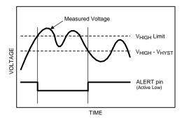
Figure 27. Alert condition cleared when measured voltage crosses V<sub>HIGH</sub> - V<sub>HYST</sub>
