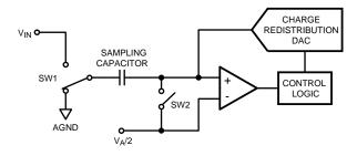
Figure 21. ADC121C021 in Hold Mode
