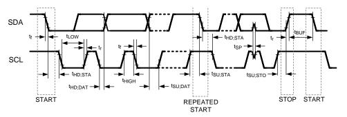
Figure 4. Serial Timing Diagram
