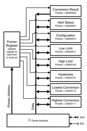
Figure 24. Register Structure
