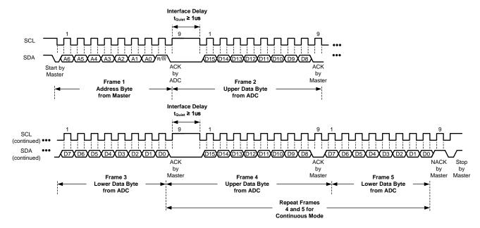
Figure 35. Reading in Quiet Interface Mode
