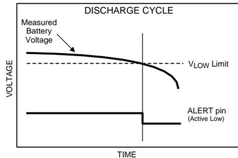
Figure 40. Discharge Cycle
