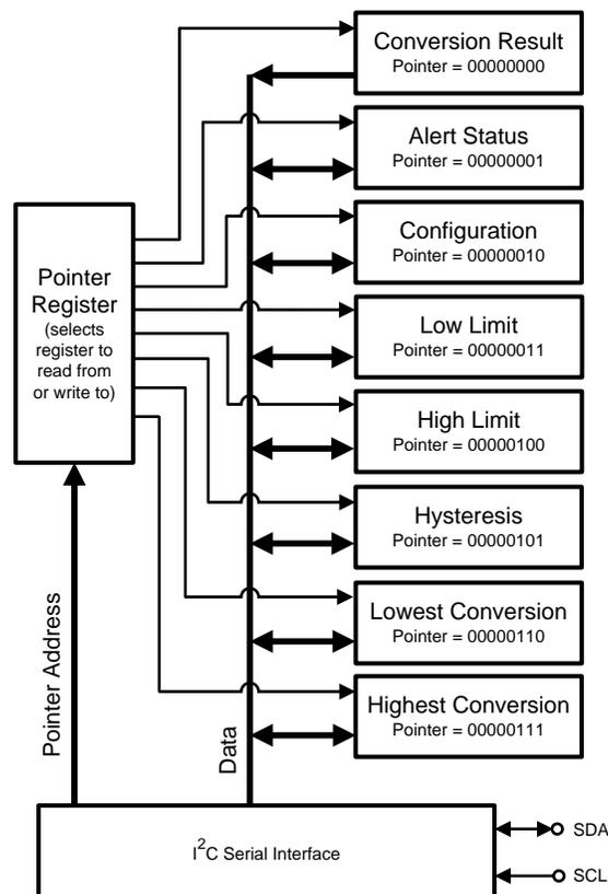
Figure 24. Register Structure
