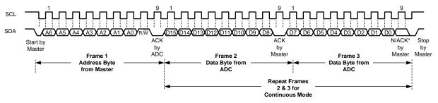
\*Note: In continuous mode, this bit must be an ACK. Immediately preceding a STOP condition, this bit must be a NACK.
