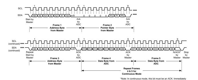
Figure 30. (b) Typical Pointer Set Followed by Immediate Read of a 2-Byte ADC Register
