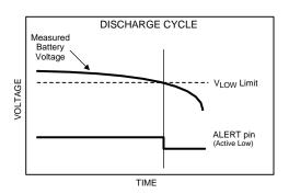
Figure 40. Discharge Cycle
