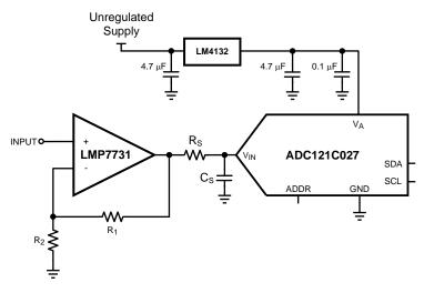
Figure 37. Buffered Input Circuit
