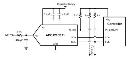
Figure 36. Typical Application Circuit
