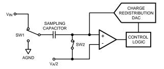
Figure 20. ADC121C021 in Track Mode
