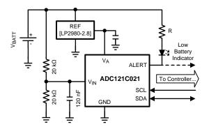
Figure 38. Intelligent Battery Monitor Circuit
