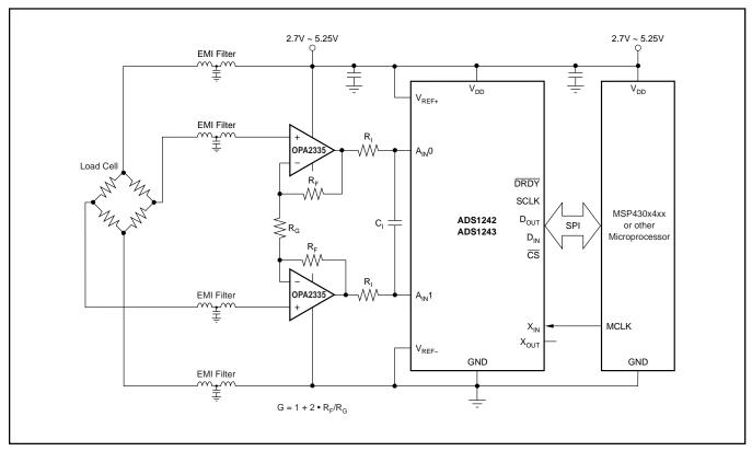
FIGURE 9. Block Diagram for a High-Precision Weight Scale.
