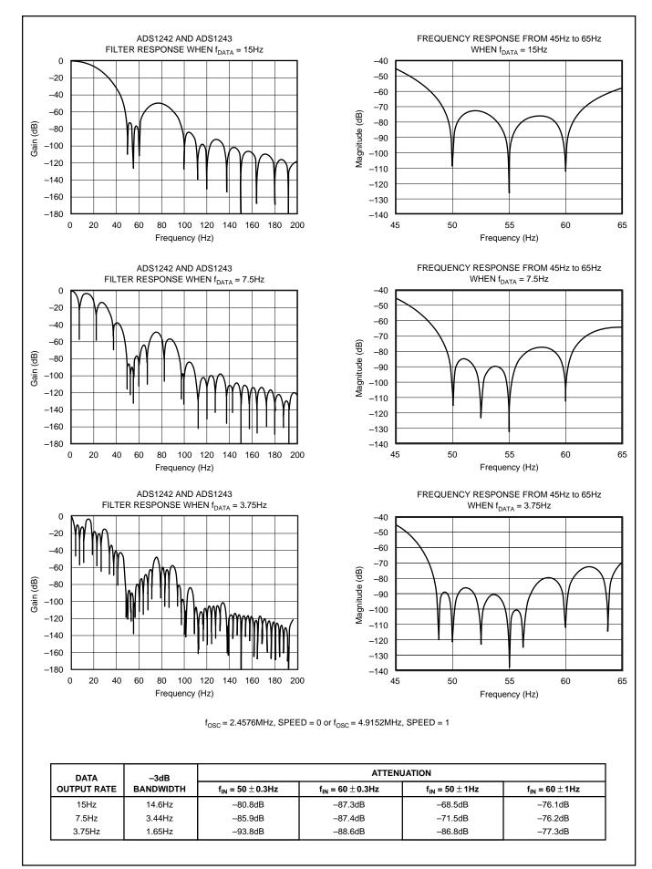
FIGURE 6. Filter Frequency Responses.
