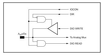
FIGURE 7. Analog/Data Interface Pin.
