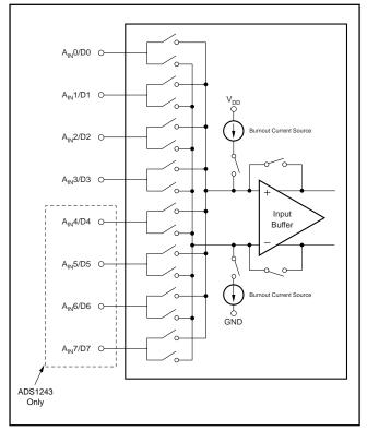
FIGURE 1. Input Multiplexer Configuration.
