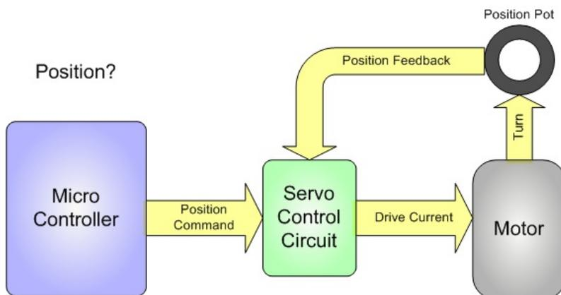
The Feedback Servos allow you to close this outer loop by providing the feedback signal to the microcontroller too!
