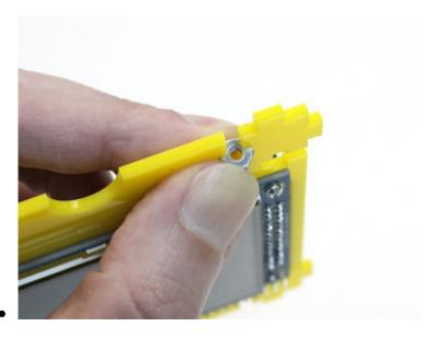
Feed a nut into the cross part of the "T," holding it in place between thumb and forefinger.
