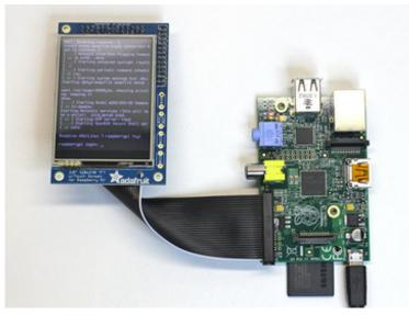
Turn the screen over and connect a USB keyboard and power. After a few seconds you should see the same bootup sequence as before.
