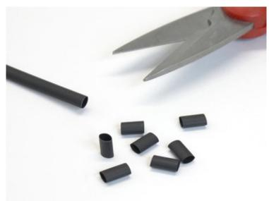
These will be used to hold wire bundles together, preventing breakage.
