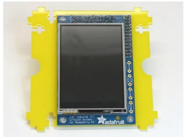
Install the PiTFT on its backing piece using three tiny #2-56 screws and matching nuts.
