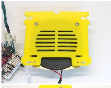
before tightening the top nuts, make sure the bottom screw holes in the speaker and grille are aligned; there's a bit of play.
