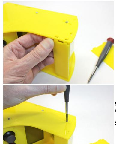
Slot the marquee into place, then re-tighten the top screw.
