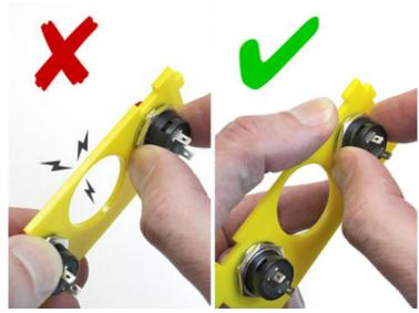
right, just flip these pieces over. Two red buttons are installed on the chosen control cutout. Because this part is thin in one spot, it must be done with care.
