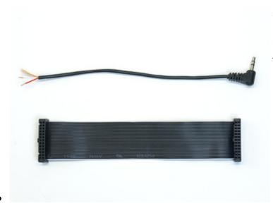
Strip about 1" of the *outer jacket* only to reveal the three wires inside: two are insulated, the third is bare copper.
