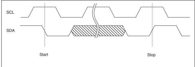
Note : The FRAM device does not need the programming wait time like twc after issuing the Stop Condition such as.
