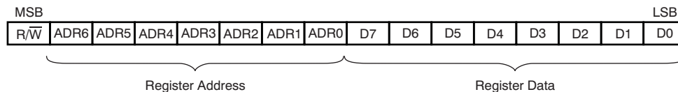
Figure 19. Control Data Word Format for MDI
