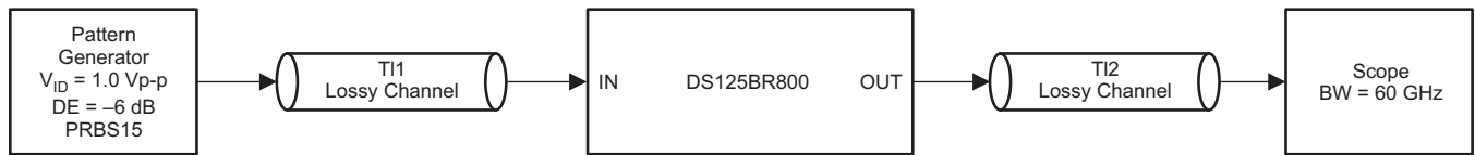
Figure 11. Test Setup Connections Diagram
