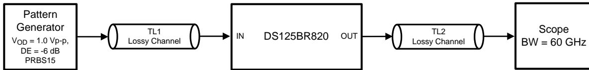
Figure 10. Test Setup Connections Diagram
