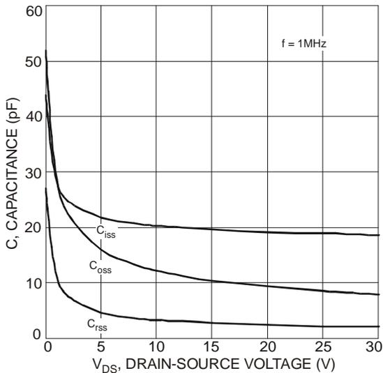
Fig. 5 Typical Capacitance
