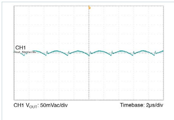
Figure 5 — Output Ripple 24V<sub>IN</sub>, 1.0V<sub>OUT</sub> at 10A
