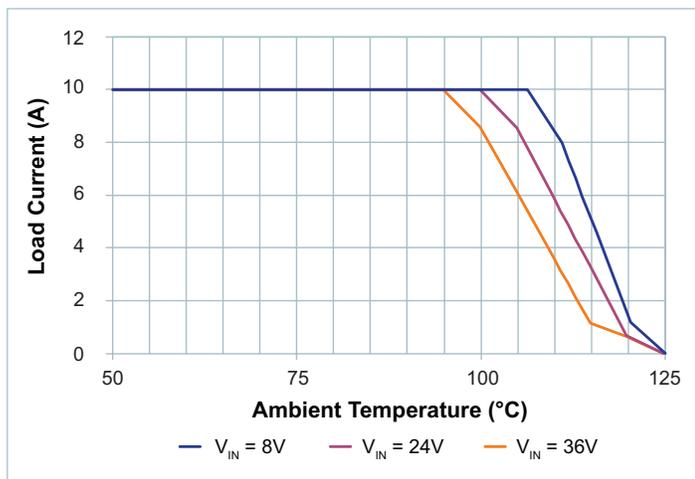
Figure 20 — Load Current vs. Ambient Temperature, 200LFM
