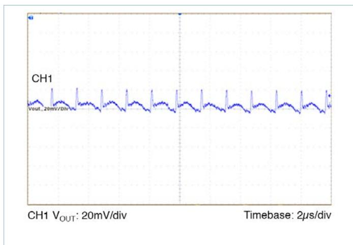
Figure 12 — Output Ripple 24V<sub>IN</sub>, 1.8V<sub>OUT</sub> at 5A
