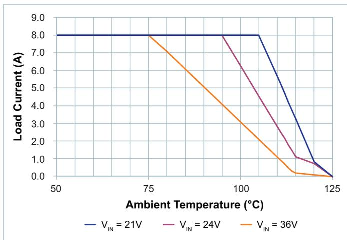
Figure 57 — Load Current vs. Ambient Temperature, 400LFM
