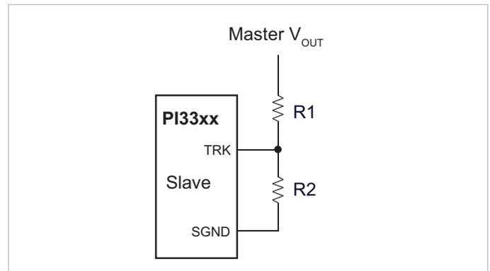
**Figure 62** — Voltage divider connections for direct tracking
