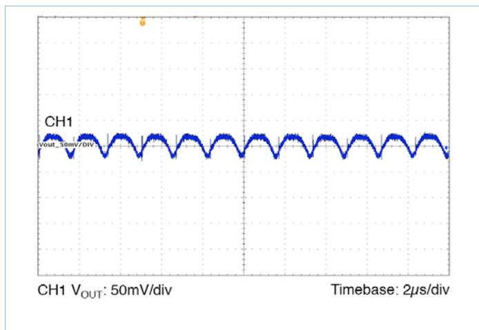
Figure 26 — Output Ripple 24V<sub>IN</sub>, 3.3V<sub>OUT</sub> at 10A
