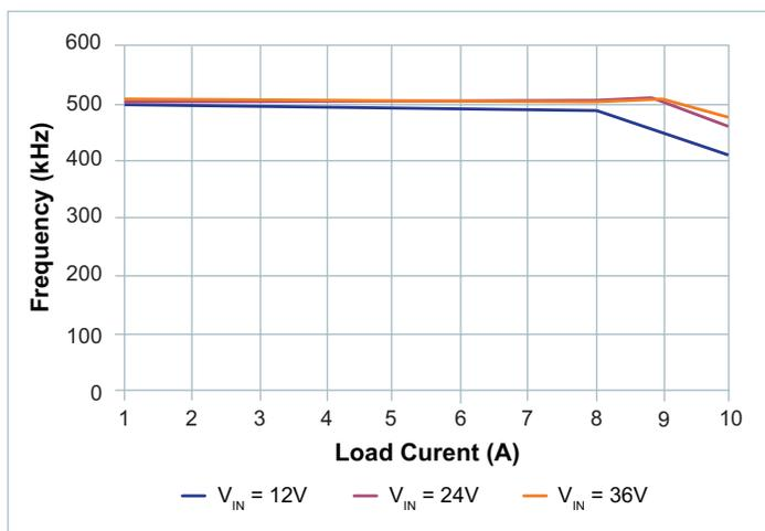
Figure 15 — Switching Frequency vs. Load Current
