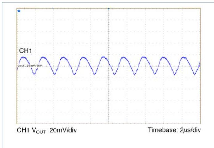
Figure 17 — Output Ripple 24V<sub>IN</sub>, 2.5V<sub>OUT</sub> at 10A
