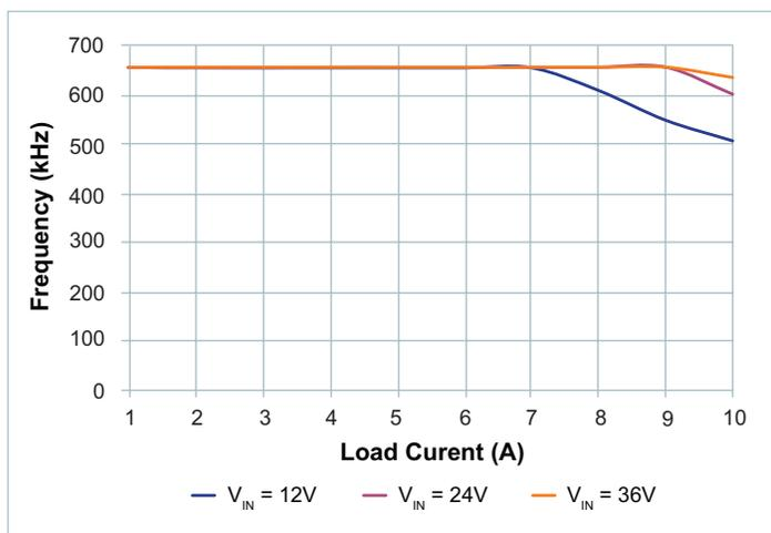
Figure 24 — Switching Frequency vs. Load Current
