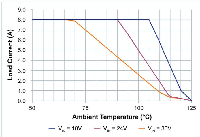
Figure 46 — Load Current vs. Ambient Temperature, 0LFM
