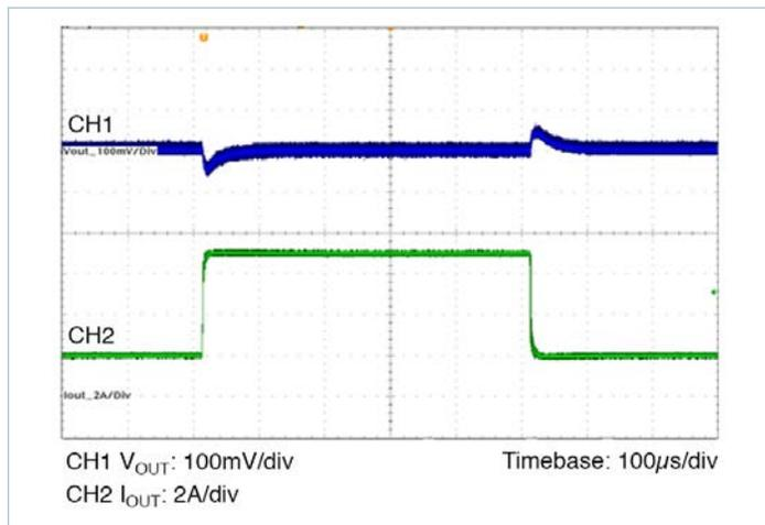
Figure 10 — Transient Response 2A to 7A, at 5A/μs
