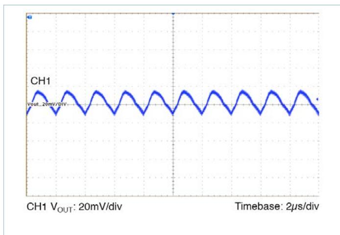
Figure 18 — Output Ripple 24V<sub>IN</sub>, 2.5V<sub>OUT</sub> at 5A
