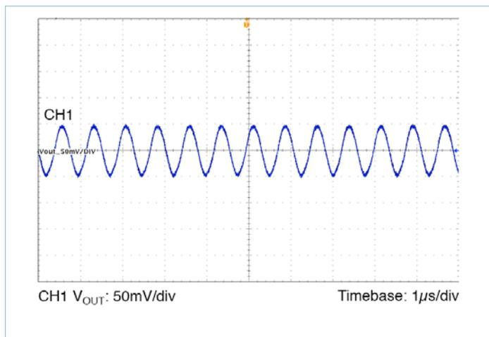
Figure 44 — Output Ripple 24V<sub>IN</sub>, 12.0V<sub>OUT</sub> at 8A
