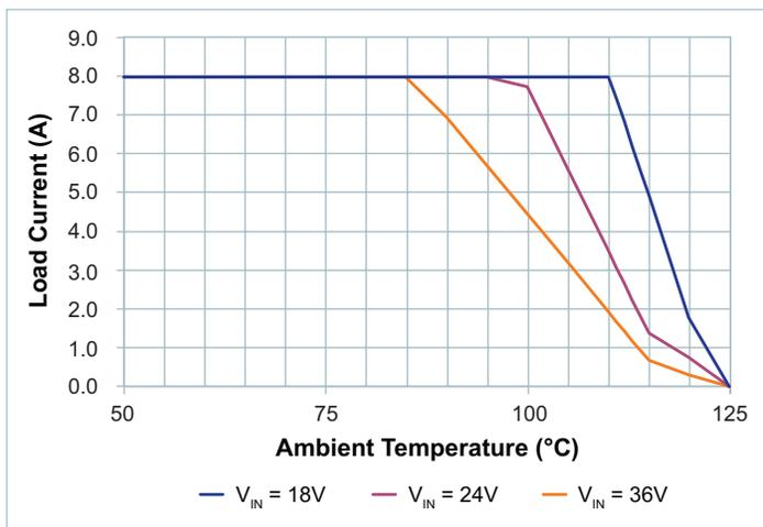
Figure 47 — Load Current vs. Ambient Temperature, 200LFM
