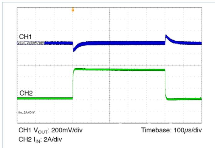
Figure 34 — Transient Response 5A to 10A, at 5A/μs
