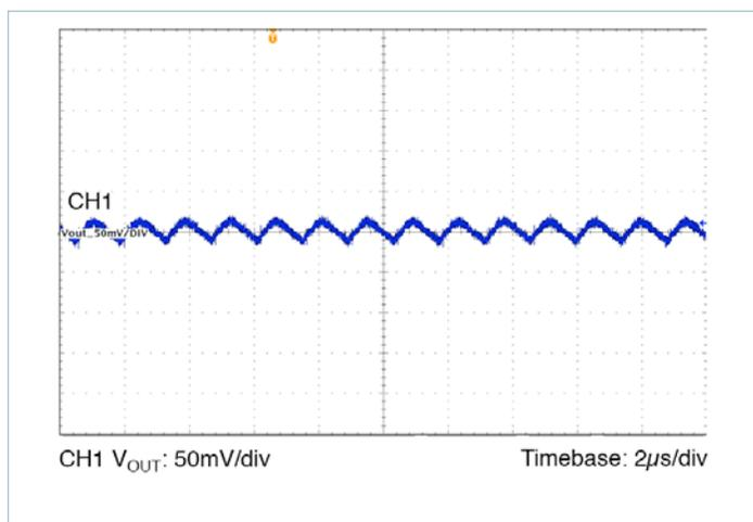
Figure 27 — Output Ripple 24V<sub>IN</sub>, 3.3V<sub>OUT</sub> at 5A
