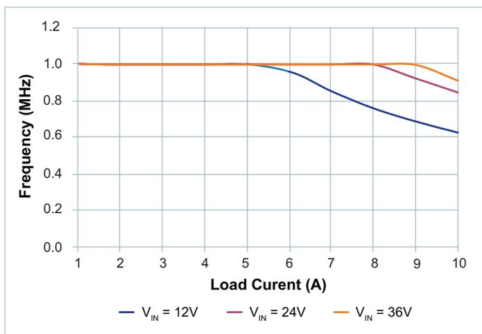
Figure 33 — Switching Frequency vs. Load Current
