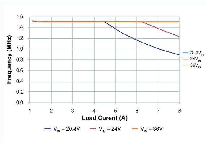
Figure 51 — Switching Frequency vs. Load Current
