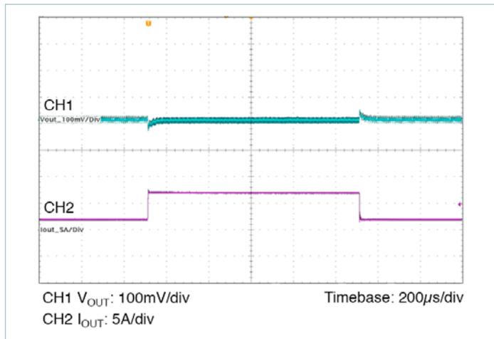
Figure 4 — Transient Response 2A to 7A, at 5A/μs
