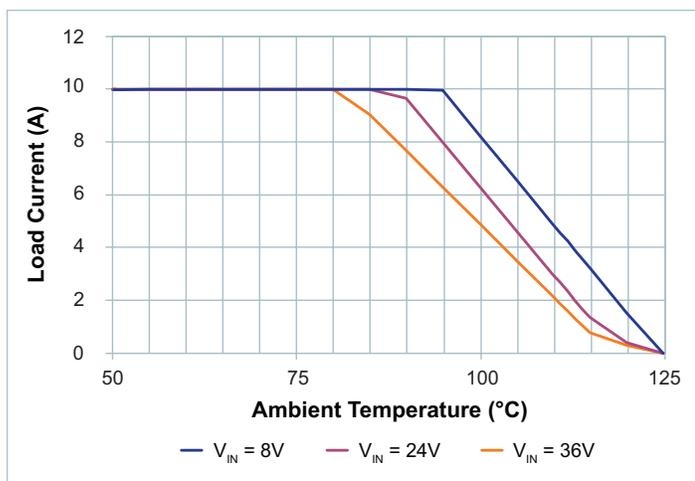
Figure 39 — Load Current vs. Ambient Temperature, 400LFM
