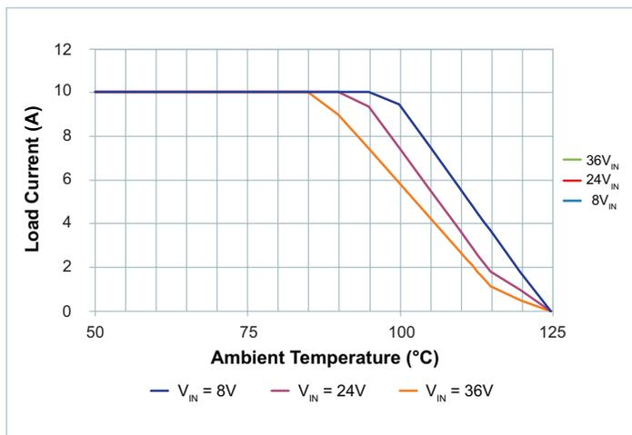
Figure 38 — Load Current vs. Ambient Temperature, 200LFM
