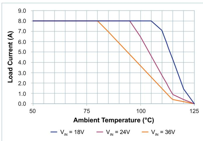
Figure 48 — Load Current vs. Ambient Temperature, 400LFM
