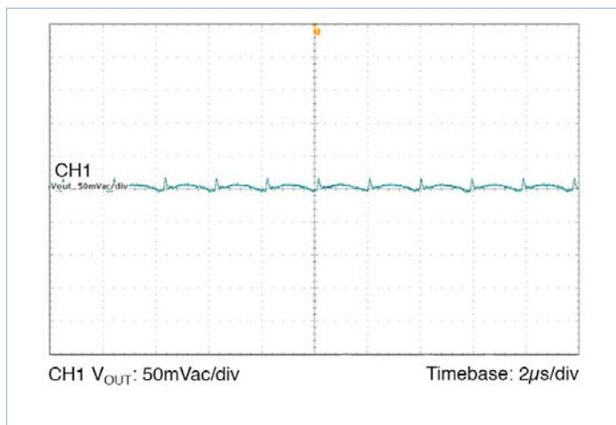
Figure 6 — Output Ripple 24V<sub>IN</sub>, 1.0V<sub>OUT</sub> at 5A
