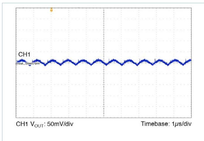
Figure 36 — Output Ripple 24V<sub>IN</sub>, 5.0V<sub>OUT</sub> at 5A
