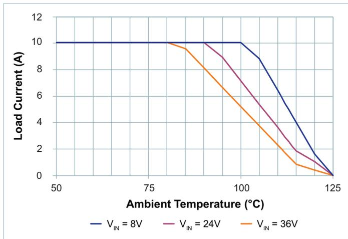
Figure 28 — Load Current vs. Ambient Temperature, 0LFM
