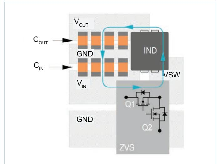
Figure 66 — Recommended component placement and metal routing
