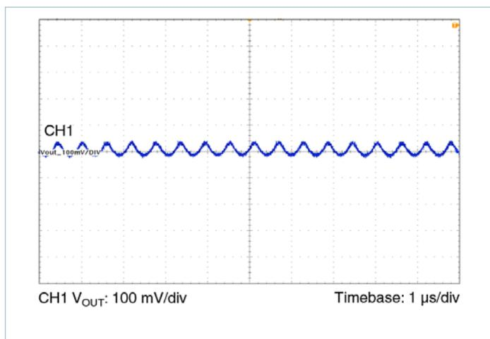
Figure 54 — Output Ripple 24V<sub>IN</sub>, 15.0V<sub>OUT</sub> at 4A
