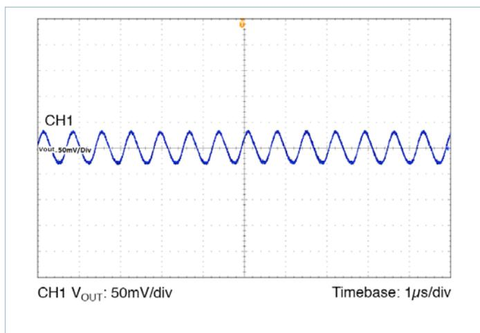
Figure 45 — Output Ripple 24V<sub>IN</sub>, 12.0V<sub>OUT</sub> at 4A
