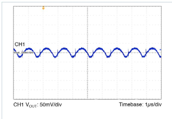
Figure 35 — Output Ripple 24V<sub>IN</sub>, 5.0V<sub>OUT</sub> at 10A
