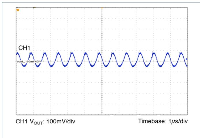
Figure 53 — Output Ripple 24V<sub>IN</sub>, 15.0V<sub>OUT</sub> at 8A
