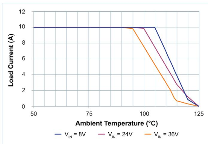
Figure 21 — Load Current vs. Ambient Temperature, 400LFM
