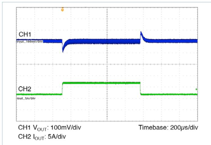
Figure 25 — Transient Response 5A to 10A, at 5A/μs
