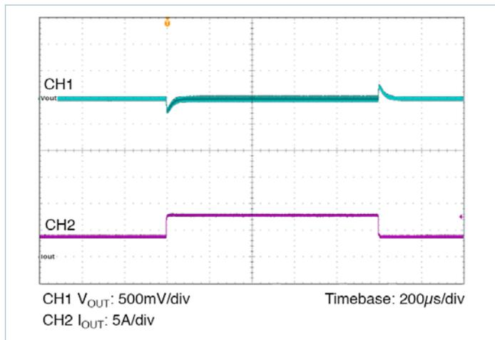
Figure 43 — Transient Response 5A to 10A, at 5A/μs
