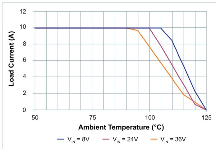
Figure 29 — Load Current vs. Ambient Temperature, 200LFM
