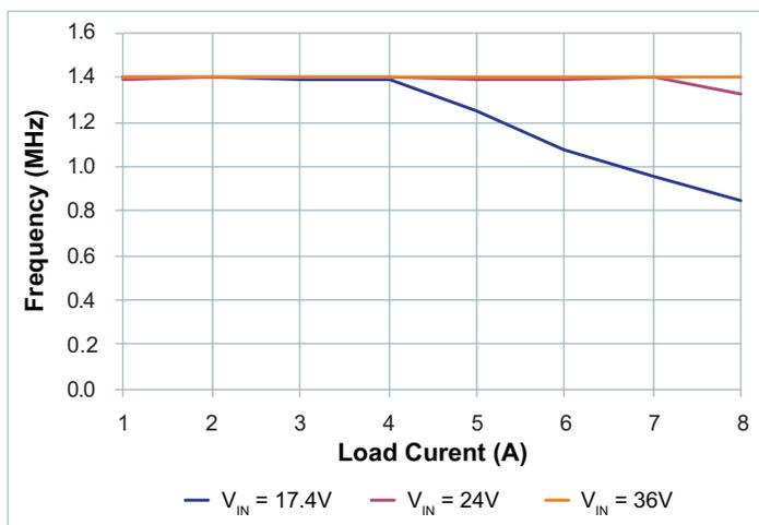
Figure 42 — Switching Frequency vs. Load Current
