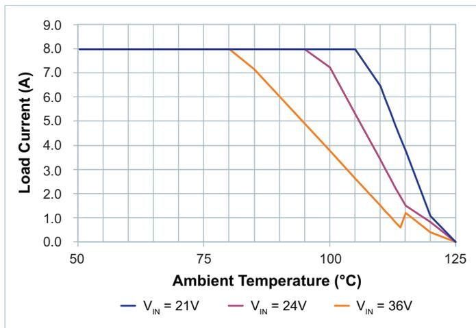
Figure 56 — Load Current vs. Ambient Temperature, 200LFM
