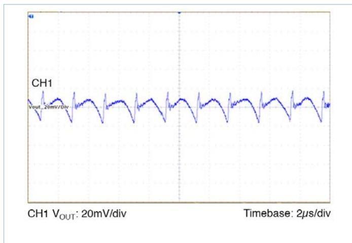
Figure 11 — Output Ripple 24V<sub>IN</sub>, 1.8V<sub>OUT</sub> at 10A
