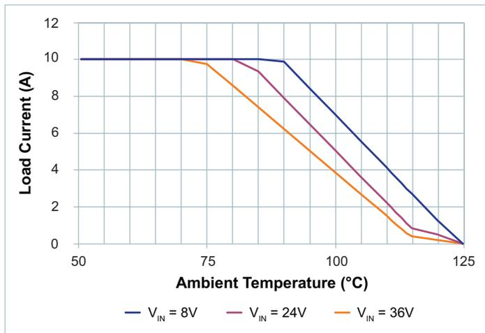
Figure 37 — Load Current vs. Ambient Temperature, 0LFM
