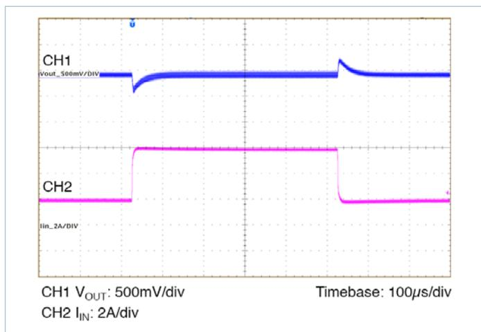
Figure 52 — Transient Response 5A to 10A, at 5A/μs
