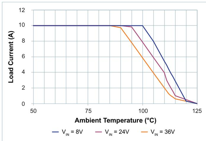
Figure 19 — Load Current vs. Ambient Temperature, 0LFM
