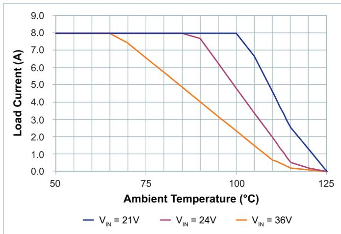
Figure 55 — Load Current vs. Ambient Temperature, 0LFM
