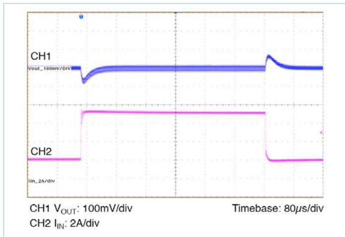
Figure 16 — Transient Response 5A to 10A, at 5A/μs
