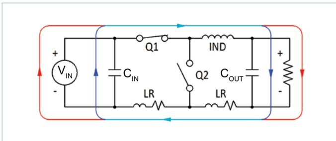
Figure 63 — Typical Buck Converter
