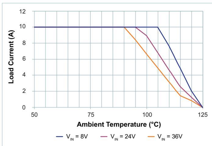
Figure 30 — Load Current vs. Ambient Temperature, 400LFM
