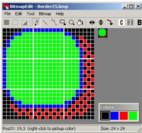
segments. This makes it necessary to keep the 8x8 size in every case. If 4-color bitmaps are used (as the preloaded border 1..20) the color can be set individually (the first color is always transparent and is not used by the eDIP). It is also possible to define full colored border (as the preloaded border for bargraphs 101...127). With the LCD-tools some sample border has been installed (see folder 'Bitmaps\Color\Border').
