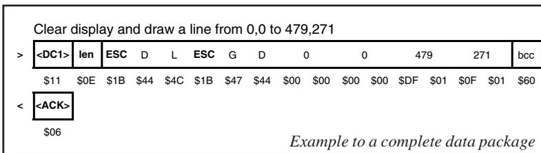
The user data is transferred framed by <DC1>, the number of bytes (len) and the checksum (bcc). The display responds with <ACK>.
