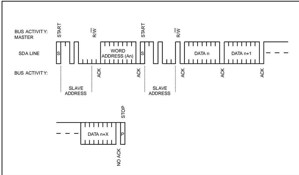
Figure 11: Alternate READ mode sequence
