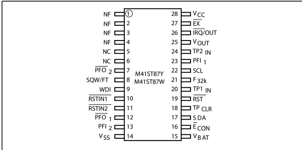
Note: No function (NF) and no connect (NC) pins should be tied to V<sub>SS</sub>. Pins 1, 2, 3, and 4 are internally shorted together.
