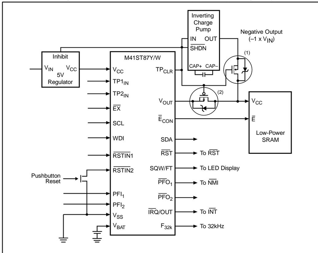
1. Most inverting charge pumps drive OUT to ground when device shut down is enabled ( $\overline{SHDN}$  = logic low). Therefore, an n-channel enhancement mode MOSFET should be used to isolate the OUT pin from the  $V_{OUT}$  of the M41ST87.
