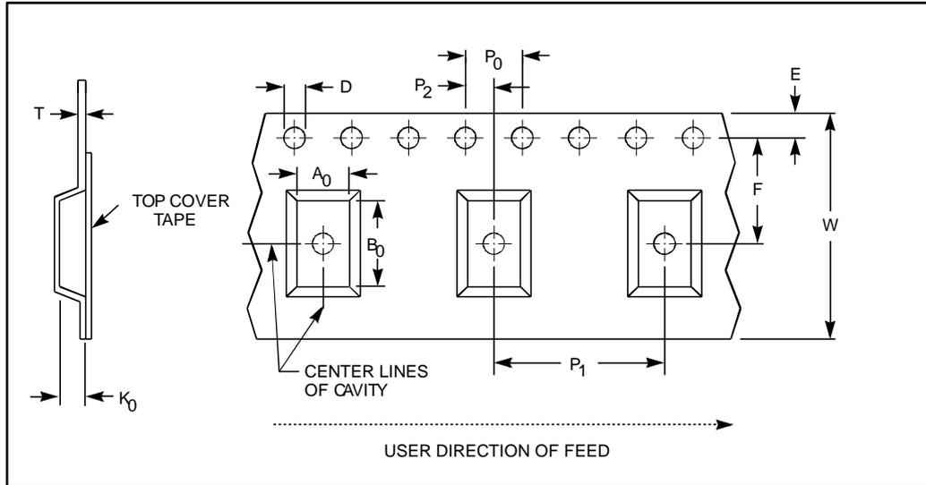
Table 24: Carrier tape dimensions for SOX28 package
