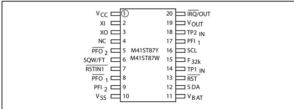
Note: No connect (NC) pin should be tied to V<sub>SS</sub>.
