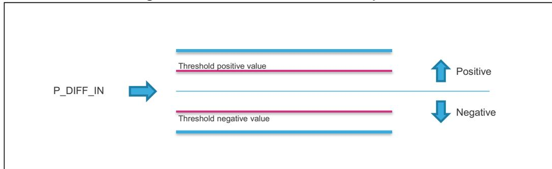
If the **AUTOZERO** bit is set to '1', the measured pressure is used as a reference on the register REF\_P (15h, 16h and 17h). From that point on, the output pressure registers PRESS\_OUT (*PRESS\_OUT\_H (2Ah)*, *PRESS\_OUT\_L (29h)* and *PRESS\_OUT\_XL (28h)*) are updated and the same value is also used for the interrupt generation:
