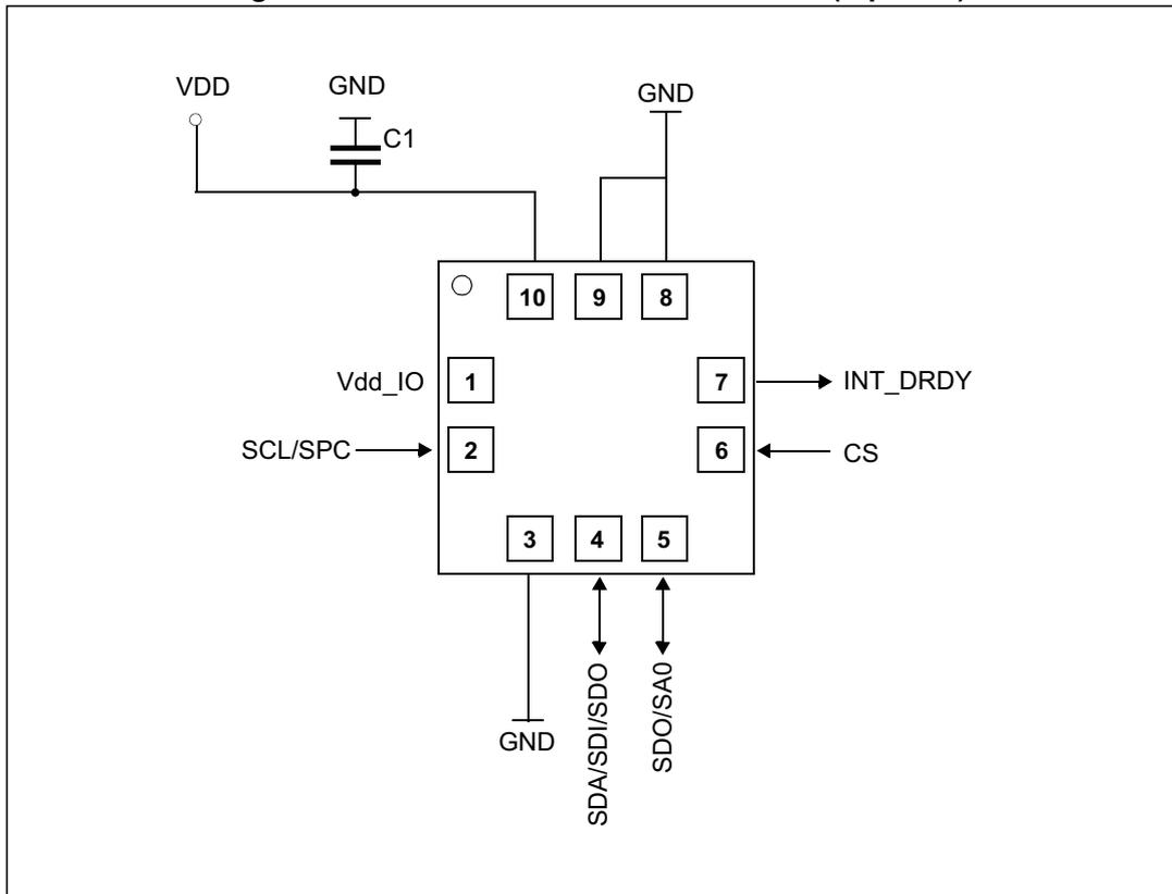
The device power supply must be provided through the VDD line; a power supply decoupling capacitor C1 (100 nF) must be placed as near as possible to the supply pads of the device. Depending on the application, an additional capacitor of 4.7  $\mu$ F could be placed on the VDD line.
