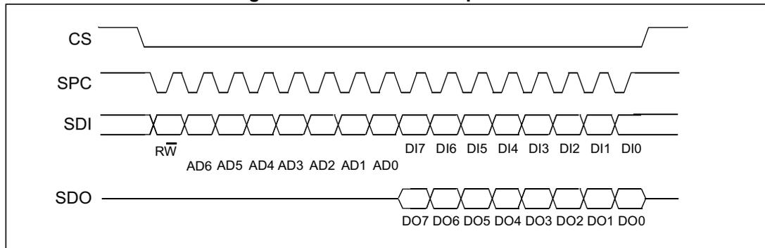
**CS** is the serial port enable and it is controlled by the SPI master. It goes low at the start of the transmission and returns to high at the end. **SPC** is the serial port clock and it is controlled by the SPI master. It is stopped high when **CS** is high (no transmission). **SDI** and **SDO** are respectively the serial port data input and output. Those lines are driven at the falling edge of **SPC** and should be captured at the rising edge of **SPC**.
