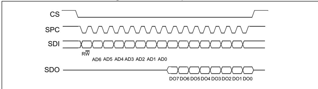
The SPI read command is performed with 16 clock pulses. The multiple byte read command is performed by adding blocks of 8 clock pulses to the previous one.
