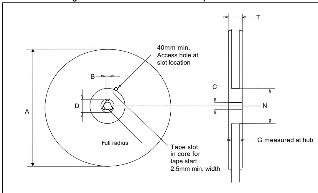
Table 22. Reel dimensions for carrier tape of CCLGA 10L package
