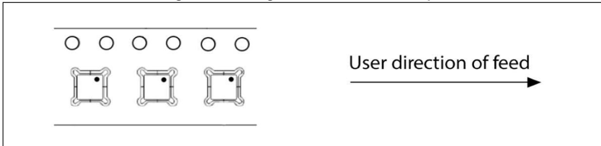
Figure 25. Reel information carrier tape CCLGA 10L
