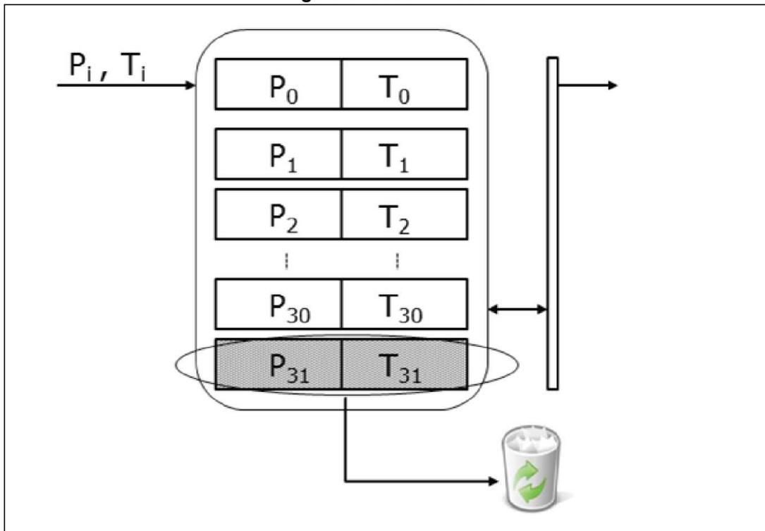
In the latter case reading all FIFO content before an overrun interrupt has occurred, the first data read is equal to the last already read in the previous burst, so the number of new data available in FIFO depends on the previous reading.
