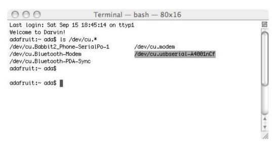
The name we are looking for is/dev/cu.usbserial-XXXX where the X's are going to be unique for each cable. Copy and paste the name into a text file so you'll remember it for later.
