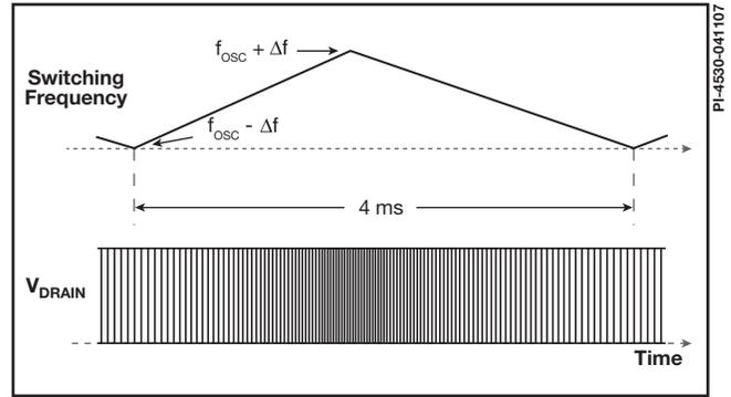
Figure 5. Switching Frequency Jitter (Idealized  $V_{DRAIN}$  Waveforms).
