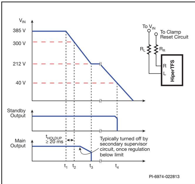
Figure 11. L and R Pin Duty Limit Mode.
