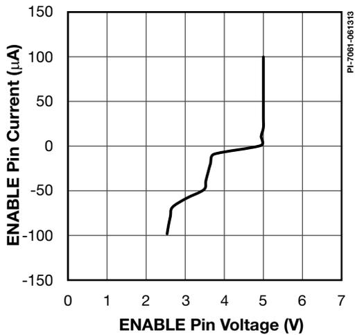
Figure 42. ENABLE (EN) Pin Current vs. Voltage.
