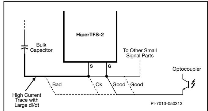
Figure 17. The PCB Trace from the Bulk Capacitor to the SOURCE Pin Contains Currents with Large  $di/dt$ . Do not Return any Small Signal Ground Connections to this Trace, Such as Small Signal Bypass Capacitors, or Optocouplers.
