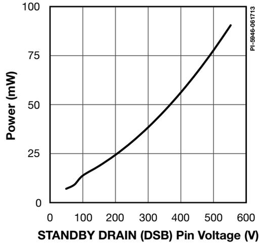
Figure 51. Standby Drain Switching Power vs. Drain Voltage.
