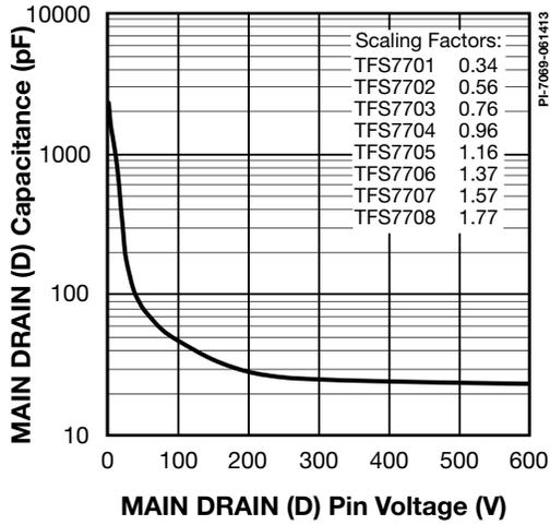
Figure 50. Main Drain Capacitance vs. Drain Voltage.
