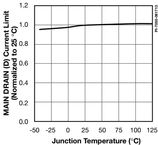
Figure 36. Main Drain (D) Current Limit vs. Temperature.
