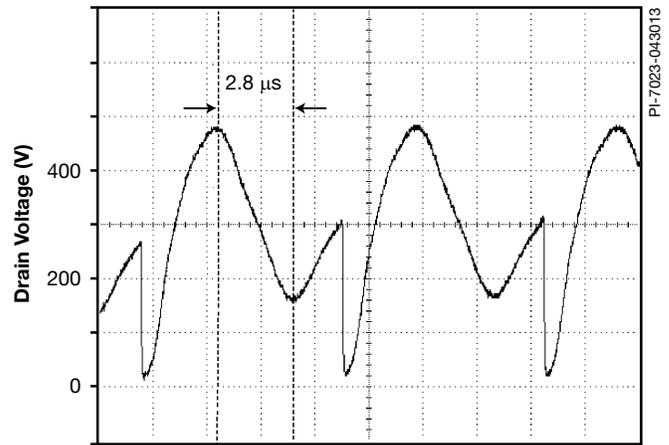
Figure 27. Drain Voltage at Zero Load, to Measure Magnetizing Resonant Frequency. In the Above Example, the Cursors Were Set to Measure a Half-Cycle. The Resonant Frequency calculates as  $f_o = 1/(2.8 \mu s \times 2) = 177 \text{ kHz}$ .
