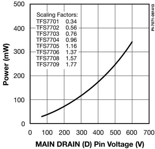
Figure 52. Main Drain Switching Power vs. Drain Voltage.
