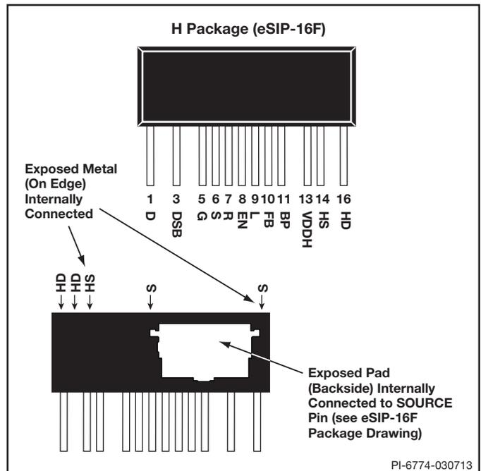
Figure 2. Pin Configuration.
