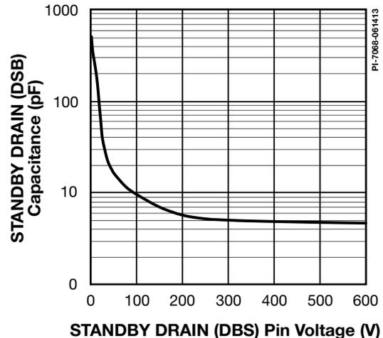
Figure 49. Standby Drain Capacitance vs. Drain Voltage.
