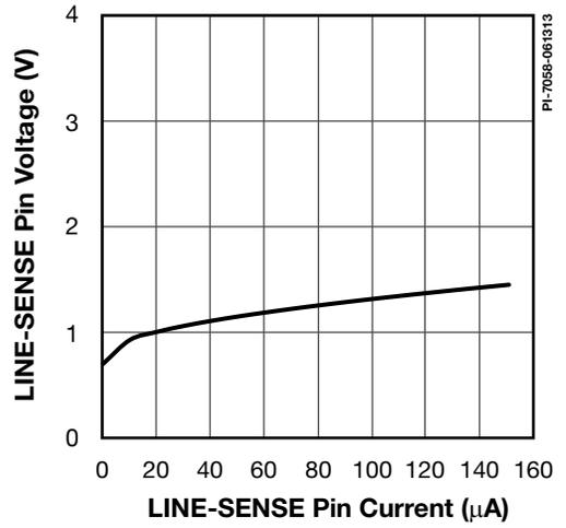
Figure 39. LINE-SENSE (L) Pin Voltage vs. Current.
