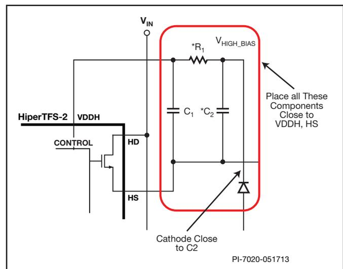
Figure 22. VDDH Components Exhibit Large  $dv/dt$  and Should be Mounted Close to the HIGH-SIDE SOURCE and VDDH pins. The Diode Should be Mounted Close to the VDDH Pin so that the Cathode Trace can be Made Short. The Anode Trace is Connected to  $V_{AUX}$  and is Quiet.
