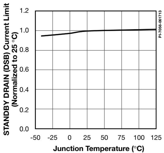
Figure 37. Standby Drain (DSB) Current Limit vs. Temperature.
