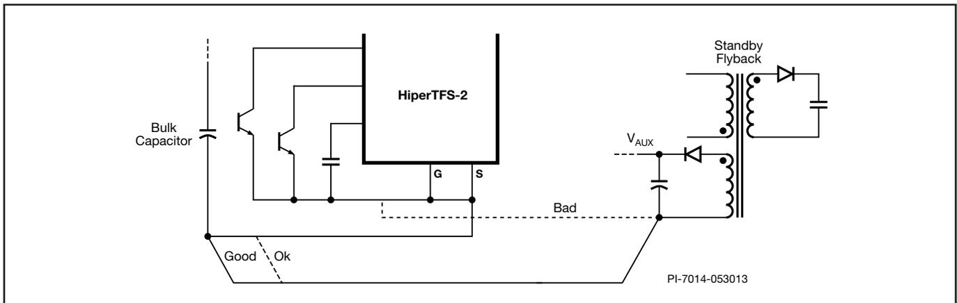
Figure 19. The (-) Terminal of the  $V_{AUX}$  Capacitor Should be Connected to B- of the Bulk Capacitor, and not to the Ground Traces. This will Improve Lightning Surge and ESD Immunity, due to Capacitive Displacement Currents Flowing Through the Primary-to-Secondary Capacitance in the Flyback Transformer.
