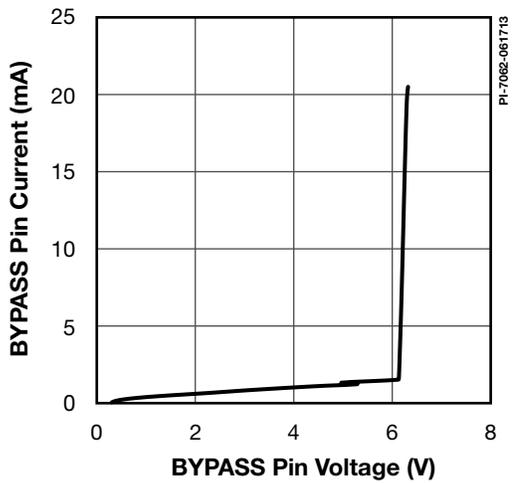
Figure 43. BYPASS (BP) Pin Current vs. Voltage.
