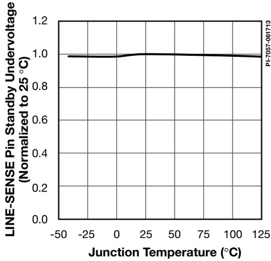
Figure 38. Standby Supply, Undervoltage Threshold vs. Junction Temperature.
