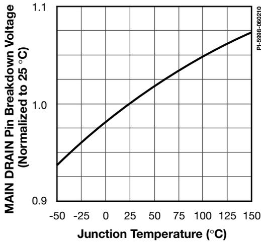
Figure 32. Main Supply, Breakdown Voltage vs. Temperature.
