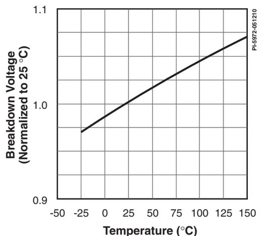
Figure 55. High-Side MOSFET Breakdown Voltage vs. Temperature.
