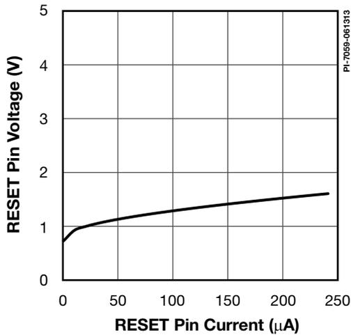
Figure 40. RESET (R) Pin Voltage vs. Current.
