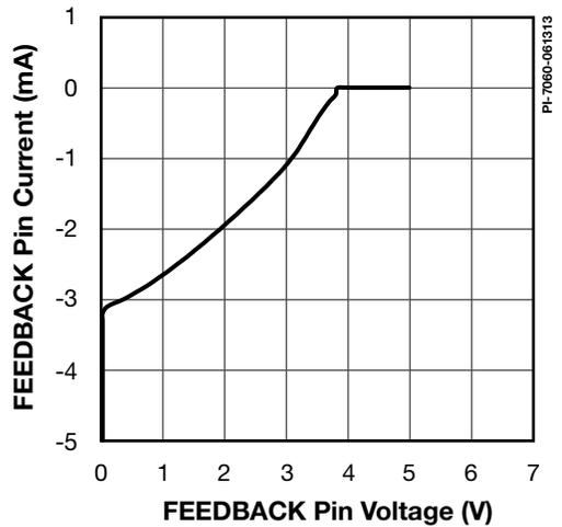
Figure 41. FEEDBACK (FB) Pin Current vs. Voltage.
