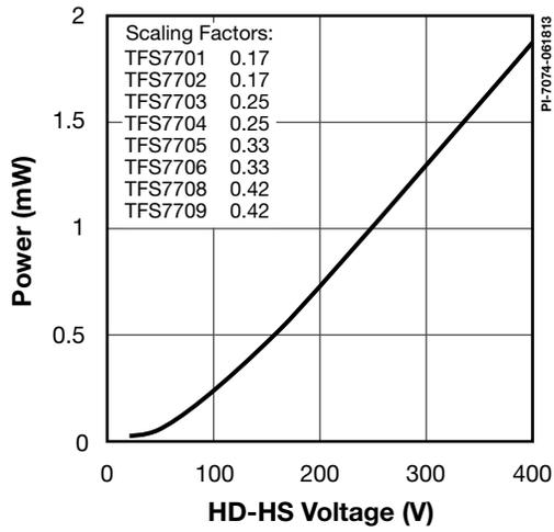
Figure 56. High-Side MOSFET (HD-HS) Power vs. Drain Voltage.
