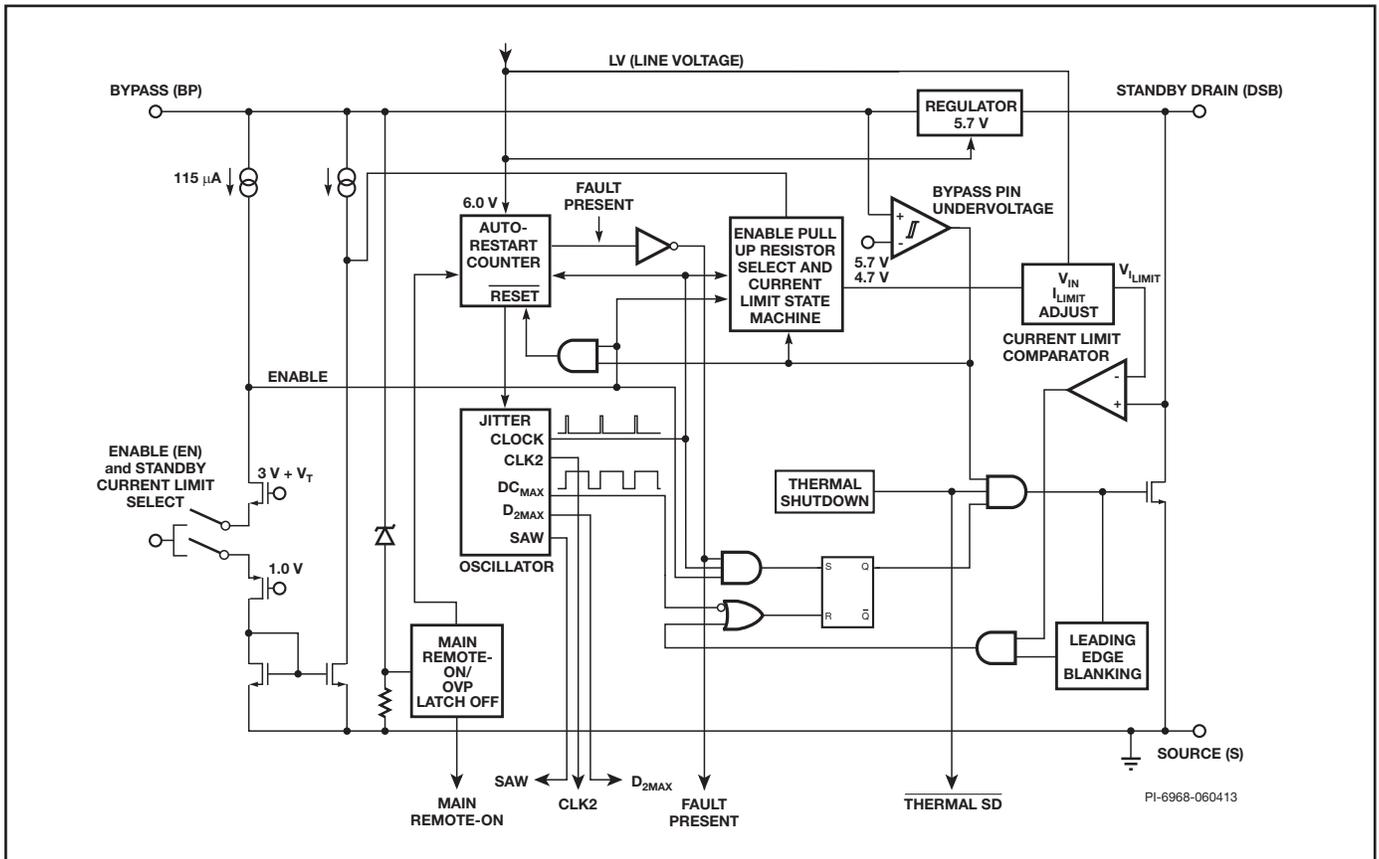
Figure 4. Functional Block Diagram for Flyback/Standby Converter.
