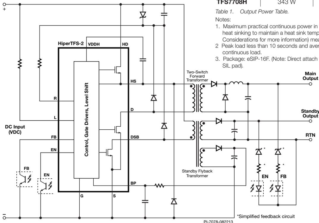
Figure 1. Schematic of Two-Switch Forward and Flyback Converter.
