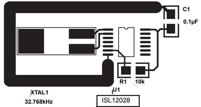
FIGURE 27. SUGGESTED LAYOUT FOR INTERSIL RTC IN SO-14
