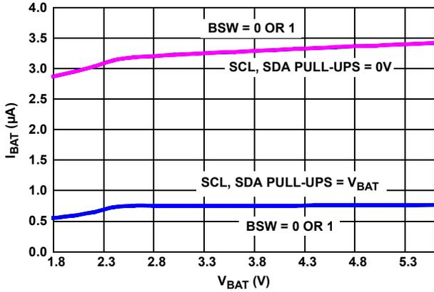
FIGURE 5.  $I_{BAT}$  vs  $V_{BAT}$ , SBIB = 0
