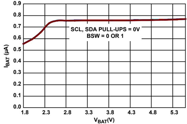
FIGURE 6.  $I_{BAT}$  vs  $V_{BAT}$ , SBIB = 1
