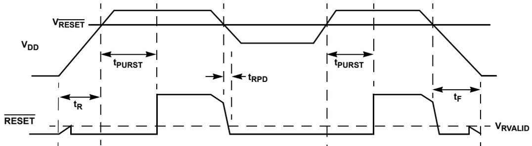
FIGURE 4. RESET TIMING
