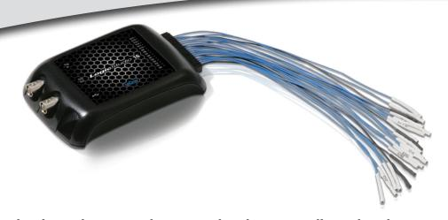
Logic analyzers are known to be slow, complicated and expensive but LogicStudio™ changes all this by delivering a powerful feature set, high-performance hardware and an intuitive point and click user-interface. With timing cursors, history mode, I²C, SPI and UART decoding, powerful triggering and simple navigation the PC is transformed in to an all-in-one debug machine.
