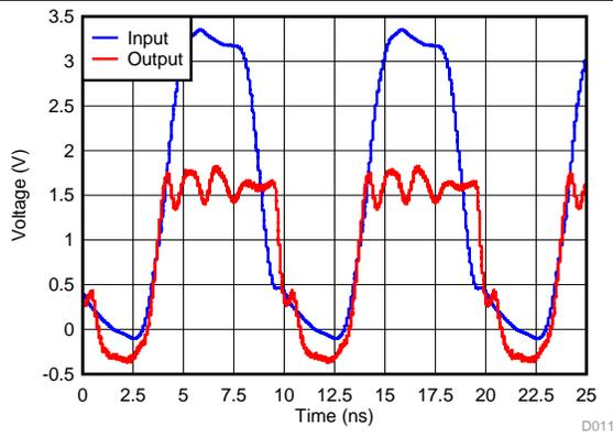
**Figure 11. Waveform From TP1 (Pull-Up Resistor: 160- $\Omega$  and 50-pF Capacitance 3.3 V to 1.8 V at 100 MHz)**
