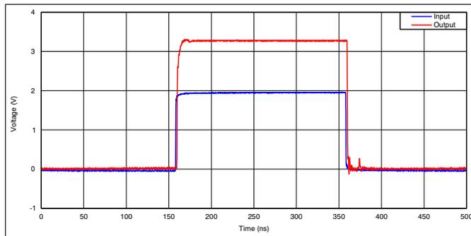
Figure 6. Captured Waveform From Above I<sup>2</sup>C Set-Up (1.8 V to 3.3 V at 2.5 MHz)
