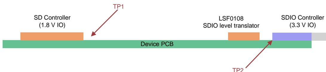
Figure 10. Device Placement
