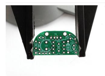
Place the PCB in a vise, and turn on the soldering iron.
