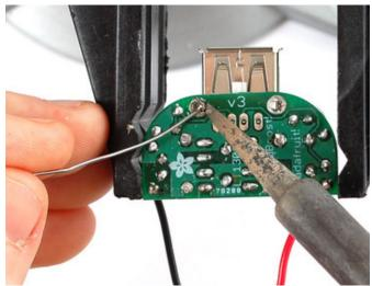
The two large side connectors are used for mechanical strength. They keep the connector attached solidly to the PCB so make sure to use lots of solder or it will break off from use.
