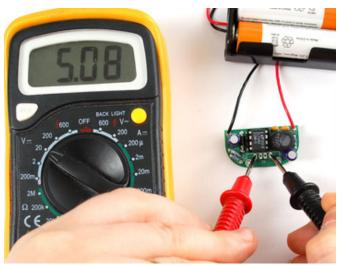
Use your multimter (hey you know how to use a multimeter right? If not, please read our voltage tutorial here (https://adafru.it/aZZ)) to measure the voltage in the two outer pins of the USB connector.
