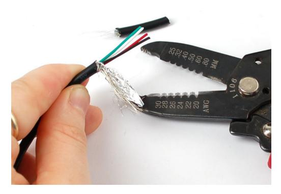
Shown above, the 4 wires. Red is power, black is ground, and the white and green wires are the data lines.
