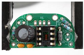
Next is the power inductor **L1**. This component is used by the DC/DC converter chip to store and convert power from low voltages to high. Inductors are just a coil of wire so they have no polarity and can be placed either way.
