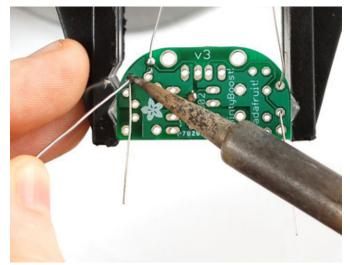
Solder the resistors as you did the 3.3K one, one point at a time, checking your work.
