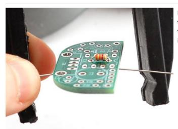
Bend the resistor into a staple and slip it onto the top of the Printed Circuit Board. Bend the little leads out so that you can flip over the PCB and the resistor will stay in place.
