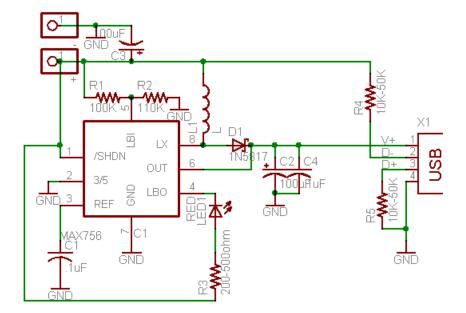
LED1, R1, R2 and R3 are optional, not included in the kit, and should be installed only if the user wants the "Low Battery Indication" function. Check the MAX756 datasheet for information on how to pick R1 and R2.
