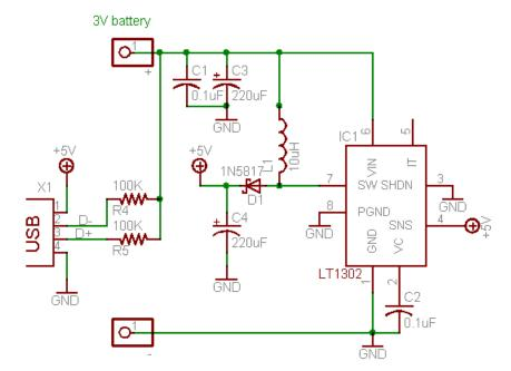
Smartphones started coming out and becoming popular, and devices with massive batteries, which meant that charging at 100mA was a no go. The mintyboost was then upgraded to the LT1302, a more expensive chip but one with a nice 500mA output ability!
