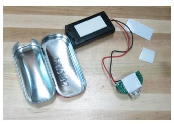
Once you're happy, remove the electronics and put the doublesided sticky foamtape on both the circuit board and the battery holder.
