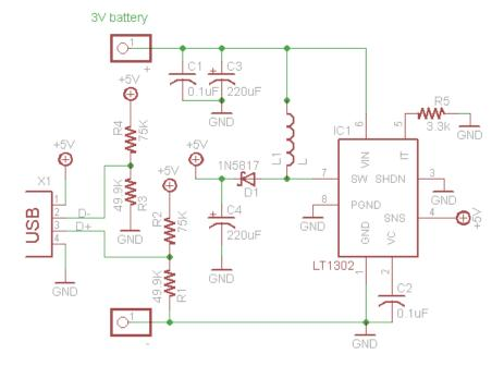
To improve compatibility with the latest smartphones and Apple devices, the charging protocol was reverse engineered so that the Mintyboost would be more universal. The pullup/down pins were also changed a full resistive divider which made it work with LiPoly batteries and Apple devices. Still uses a LT1302 chip.
