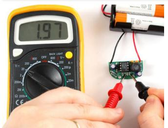
Next check between the rightmost pin and the second and third pin. They should both be at just about 2.0V
