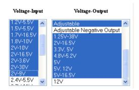
Looking over this list, it looks like I have a lot of options so I'm going to go back and select only the chips that can be preset to 5V (as opposed to adjustable ones that use 2 resistors to set the voltage). 5V is very common so every reasonable DC/DC chip will be available with such an option.
