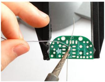
Now you'll solder! Place the flat of the soldering iron tip against the silver ring (pad) and one of the wires of the resistor (lead) at the same time for 2 seconds. This will heat them both up to 600-700 degrees. Then poke the end of the solder so that it flows into the hole and forms a solder joint.
