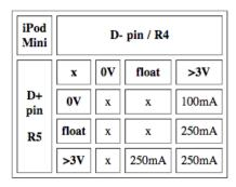
OK, so yes when the pins are floating no charging occurs. The next thing to note is that whether the pins are pulled up or down effects the current draw. Since this was the first Mintyboost, using the MAX756, we wanted to use the lower 100mA rate so one pin pulled down and another pulled up. This would be more efficient for the battery use and keep the chip from getting hot (it could provide 250mA but didn't like it much).
