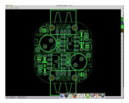
I always check the boards with <a href="https://www.freedfm.com">www.freedfm.com</a> before I ship them off to be made. I used 4pcb.com so it's the same company but even if you don't go with 4pcb.com as your PCB manufacturer, it's a neat service.
