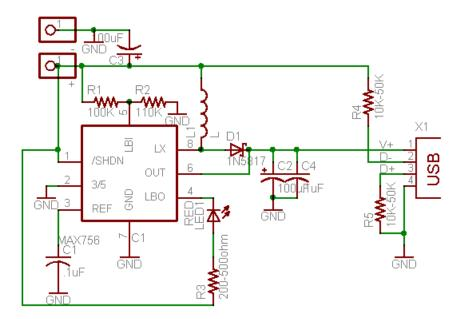
After a few months it became clear that some devices especially Apple music players, needed pullup/down resistors, so a new version that could fit 1 pullup and 1 pulldown was designed. This version still used the MAX756.
