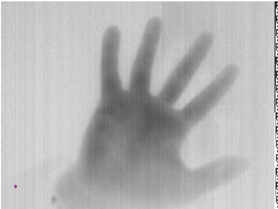
Figure 8 : Raw tap A phase0 image of a hand with enabled test columns
