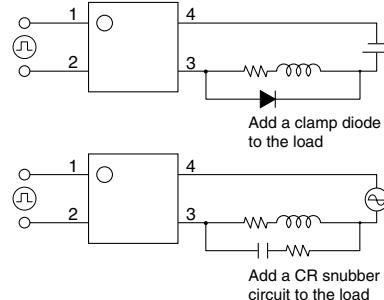
2) Even if spike voltages generated at the load are limited with a clamp diode if the circuit wires are long, spike voltages will occur by inductance. Keep wires as short as possible to minimize inductance.
