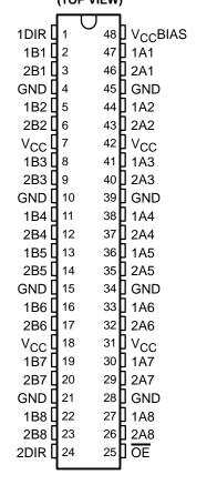
one 16-bit transceiver. They allow data transmission from the A bus to the B bus or from the B bus to the A bus, depending on the logic level at the direction-control (DIR) input. The output-enable (OE) input can be used to disable the device so that the buses are effectively isolated. When  $\overline{OE}$  is low, the device is active.
