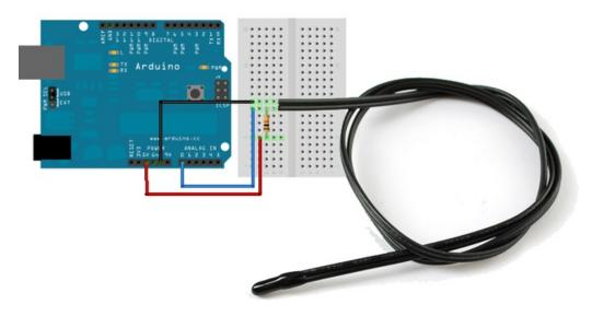
Connect one end of the 10K resistor to 5V, connect the other end of the 10K 1% resistor to one pin of the thermistor and the other pin of the thermistor to ground. Then connect Analog 0 pin to the 'center' of the two.
