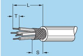
**Note:** the tolerances on these dimensions are: L:  $\pm 0.5$  mm; S:  $\pm 0.5$  mm; T:  $\pm 0.2$  mm.
