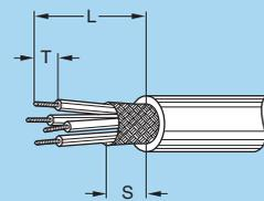
**Note:** <sup>1)</sup> center wire L = 16.5. <sup>2)</sup> center wire L = 20.5. <sup>3)</sup> 5 center wires L = 20.5.
