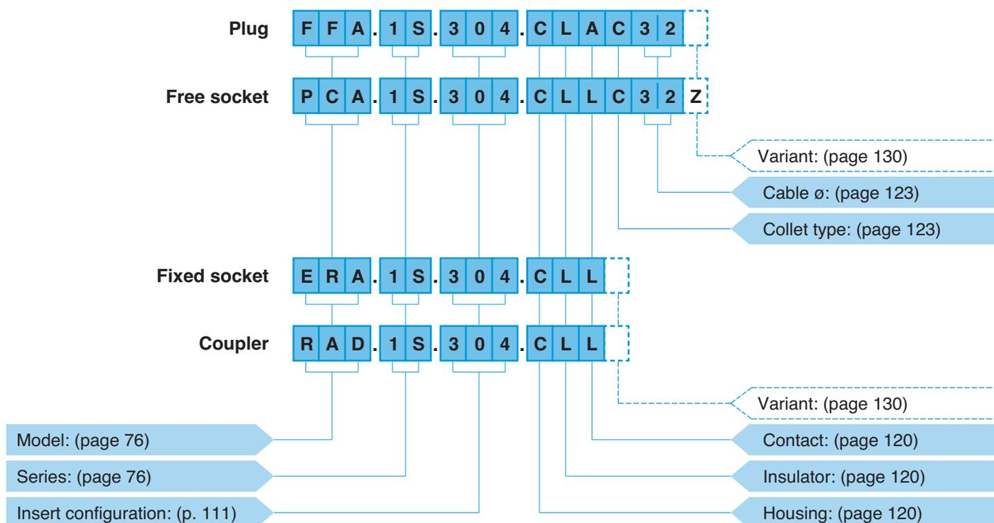
**FFA.1S.304.CLAC32** = straight plug with cable collet, 1S series, multipole type with 4 contacts, outer shell in chrome-plated brass, PEEK insulator, 2 male and 2 female solder contacts, C type collet for a 3.2 mm diameter cable.
