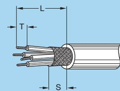
**Note:** <sup>1)</sup> In 0B and 1B series, «L» and «S» dimensions shall be increased by 2 mm for the largest collet (D56 in 0B series; D76 in 1B series). The tolerances on these dimensions are: L: ± 0.5 mm; S: ± 0.5 mm; T: ± 0.2 mm.
