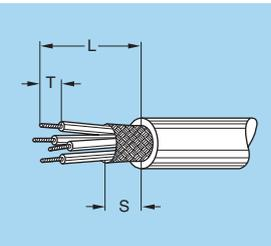
**Note:** the tolerances on these dimensions are: L: ± 0.5 mm; S: ± 0.5 mm; T: ± 0.2 mm.
