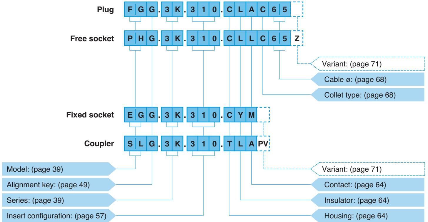
**FGG.3K.310.CLAC65** = straight plug with key (G) and cable collet, 3K series, multipole type with 10 contacts, outer shell in chrome-plated brass, PEEK insulator, male solder contacts, C type collet for 6.5 mm diameter cable.
