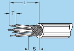
**M5** elbow plugs (90°) with cable collet, clamping type D or M (solder or crimp contacts)
