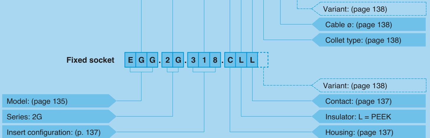
**FGG.2G.318.CLAD52** = straight plug with cable collet, 2G series, multipole type with 18 contacts, outer shell in chrome-plated brass, PEEK insulator, male solder contacts, D type collet for 5.2 mm diameter cable.
