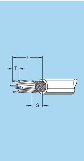
**Note:** <sup>1)</sup> In 1B series, «L» and «S» dimensions shall be increased by 2 mm for the largest collet (D76 in 1B series). In 5B series, «L» and «S» dimensions shall be increased by 13 mm for the largest collet (D25). <sup>2)</sup> Crimp contacts are available only for connectors fitted with male contacts. The tolerances on these dimensions are: L: ± 0.5 mm; S: ± 0.5 mm; T: ± 0.2 mm.
