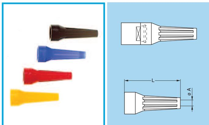
A bend relief made from thermoplastic polyurethane elastomer can be fitted over LEMO plugs and sockets that are supplied with nut for fitting such bend relief. They are available in nine different colours match with the GRA insulating washers (see page 171). Use the part numbers shown below to order this accessory separately.
