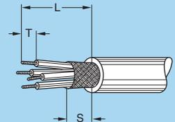
**Note:** <sup>1)</sup> crimp contacts are available only for connectors fitted with male contacts. The tolerances on these dim. are: L: ± 0.5 mm; S: ± 0.5 mm; T: ± 0.2 mm.
