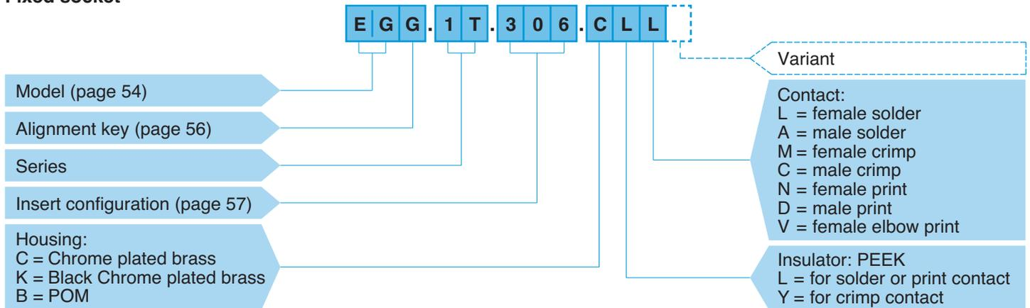
**EGG.1T.306.CLL** = fixed socket, nut fixing, with key (G), 1T series, multipole type with 6 contacts, outer shell in chrome-plated brass, PEEK insulator, female solder contacts.
