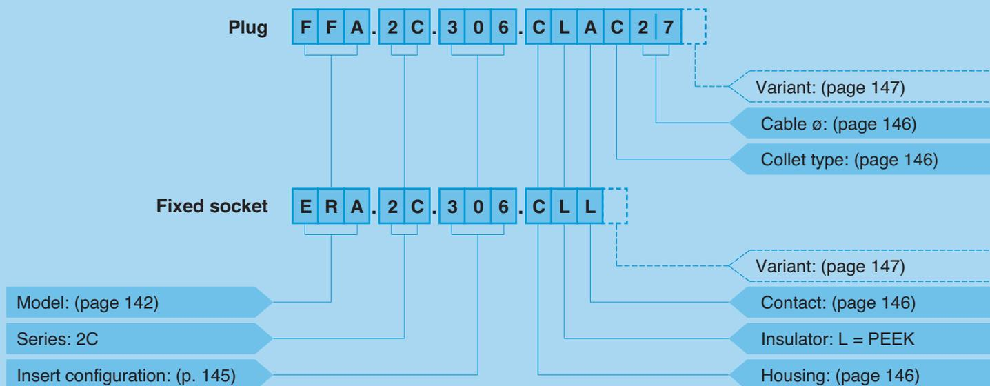
**FFA.2C.306.CLAC27** = straight plug with cable collet, 2C series, multipole type with 6 contacts, outer shell in chrome-plated brass, PEEK insulator, male solder contacts, C type collet for 2.7 mm diameter cable.
