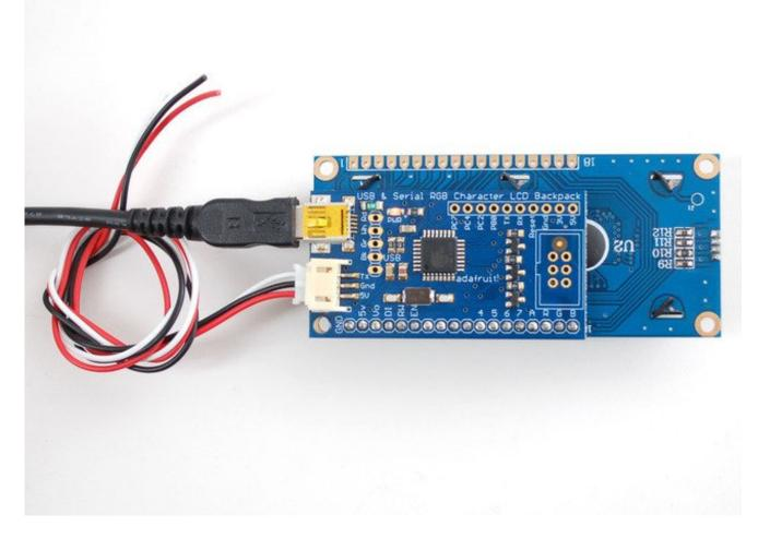
You can also connect with the TTL serial input. This is the red/black/white cable. Power is provided by connecting the black wire to ground and the red wire to +5V. The white cable is the 5V TTL serial input. By default, the backpack is configured for 9600 baud, 8 bit, no
