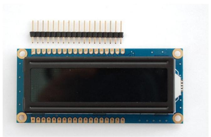
Place the header with the long side down into a breadboard. then place the LCD on top. If you're using an LCD with two rows available, make sure you're using the row that matches the image below.
