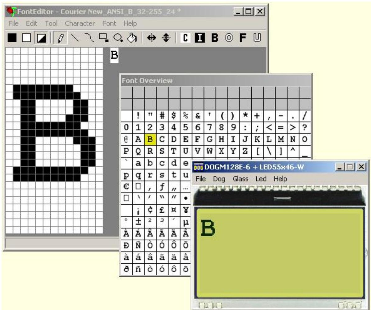
All graphic displays from ELECTRONIC ASSEMBLY EA DOG series do provide a full graphic memory. To display some characters and text, a small bitmap needs to be written into this graphic memory. The FontEditor from ELECTRONIC ASSEMBLY generates those bitmap files. It will be included in  $\mu\text{C}$  sourcefiles then.
