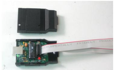
Plug in the two cables as shown, the red stripes on top and so that the cables don't bend over the plug (the case wont fit).
