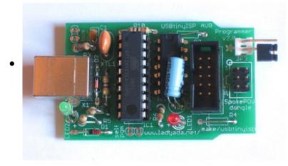
If you're not using the USBtiny to talk to a SpokePOV kit, and if you are using a target that has some load on the SCK and MOSI pins, you may need to replace R4 and R7 with jumpers as the 1.5K resistors will have trouble driving the load!
