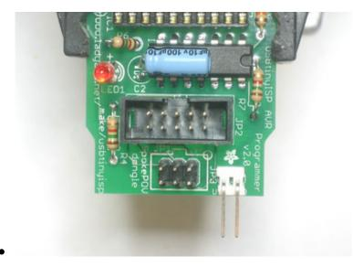
Almost done! The last set of parts are the headers for the cables, and the jumper header. The 10-pin box header has a notch in it, make sure it matches up with the silkscreen, as shown.
