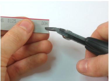
with 10-conductor wire. (The kit ships with 6-conductor) If so, just use your diagonal cutters (or a knife) to cut a notch so that the red stipe is on the 6-conductor side.
