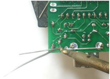
Solder and clip the two LEDs.
