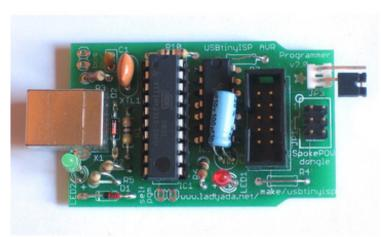
do the remaining 5 all at once. Place **R10** (10K pullup resistor), **R3**, **R5** and **R6** (1.5K resistors for the USB connection, LEDs and output buffer).
