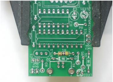
The first part to solder is a resistor, **R1**. This resistor has a 470hm value, check the parts list to make sure you have the right one. Bend the two legs of the resistor so that its staple-shaped. Then slide the resistor into the PCB so that the outline matches the image on the silkscreen. Resistors are bi-directional so you don't have to worry about putting it in the wrong way.
