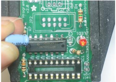
sure the longer leg of the capacitor goes into the hole with a +. Bend the capacitor so that it lies on top of the buffer chip.
