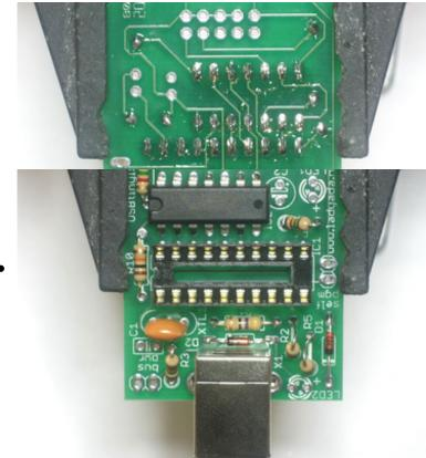
Next is the USB connector and the 12.00MHz ceramic oscillator. The USB connector is what we use to plug into the computer, the oscillator makes sure the USBtiny microcontroller runs at the precise rate necessary to communicate at the very picky USB protocol rates.
