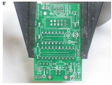
Next, get ready by placing the PCB in a vise so that you can easily place and solder the parts in!
