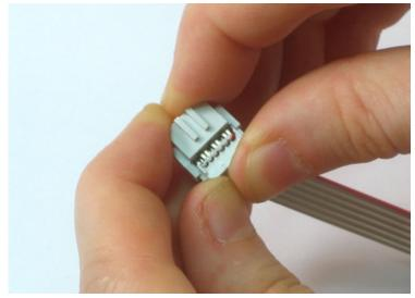
Get it started by just squeezing it with your fingers to make sure the wires are aligned properly. You wont be able to finish the cable this way so don't try!
