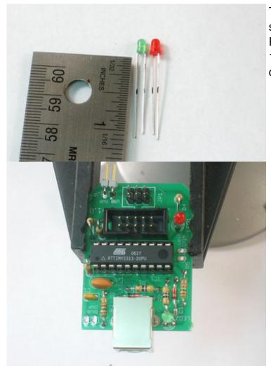
The two LEDs are next. They should stand-off a bit from the PCB so make a marking about 1/2" (1cm) from where the colored plastic ends.
