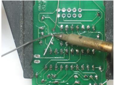
Solder and clip both capacitor's leads.
