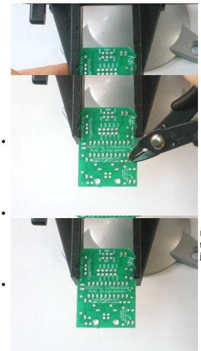
Use the diagonal cutters to clip the legs off just above the solder joint.
