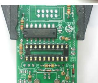
Next to be placed is the 74AHC125 buffer. This chip does a level-shifting conversion on signals from the USBtiny microcontroller to the device being programmed. This way you can safely program chips that vary from 1.8V to 5.5V voltage.
