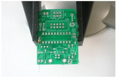
Place the first component: the 10K resistor as shown. Resistors are non-directional, so you can put them in 'either' way and they'll work fine. When you put the legs through the PCB, bend them out so when the PCB is flipped it wont fall out.
