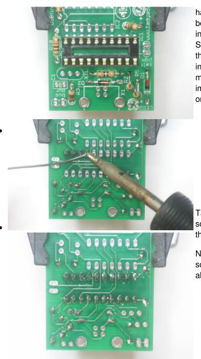
hard work. A socket is useful because you can replace the chip in case of upgrade or damage. Sockets have a little notch in them to indicate which way to put in the chip. This notch should match the notch in the silkscreen image, in this picture, the notch is on the left-hand side.
