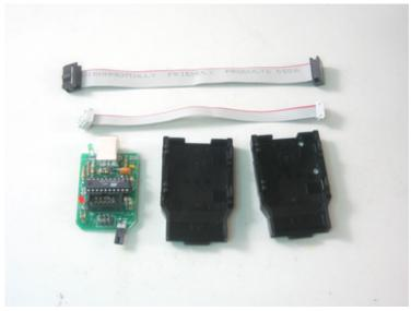
Take the PCB, two case halves and the cables you've made.
