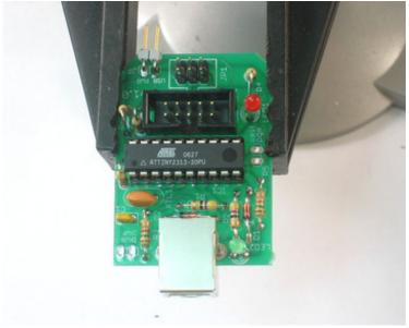
Soldering's done. Next up, insert the microcontroller. You can do this by gently bending the legs in using your fingertips or the tabletop.
