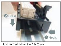
2. Press the Unit onto the DIN Track to secure it.
