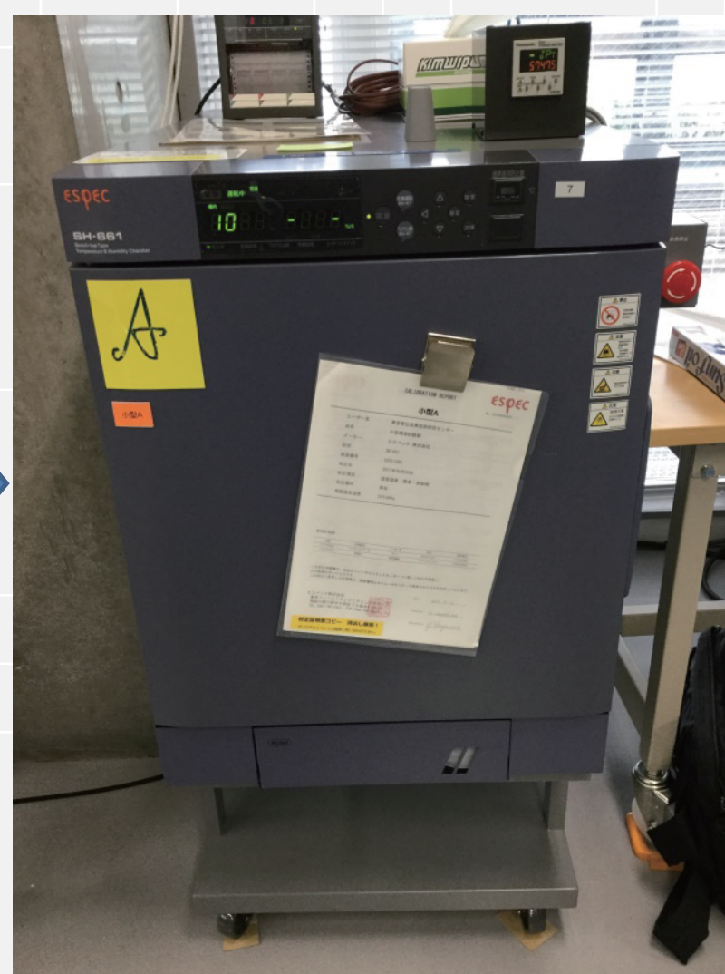
ESPEC Model SH-661 Thermostat 1hour 100℃
